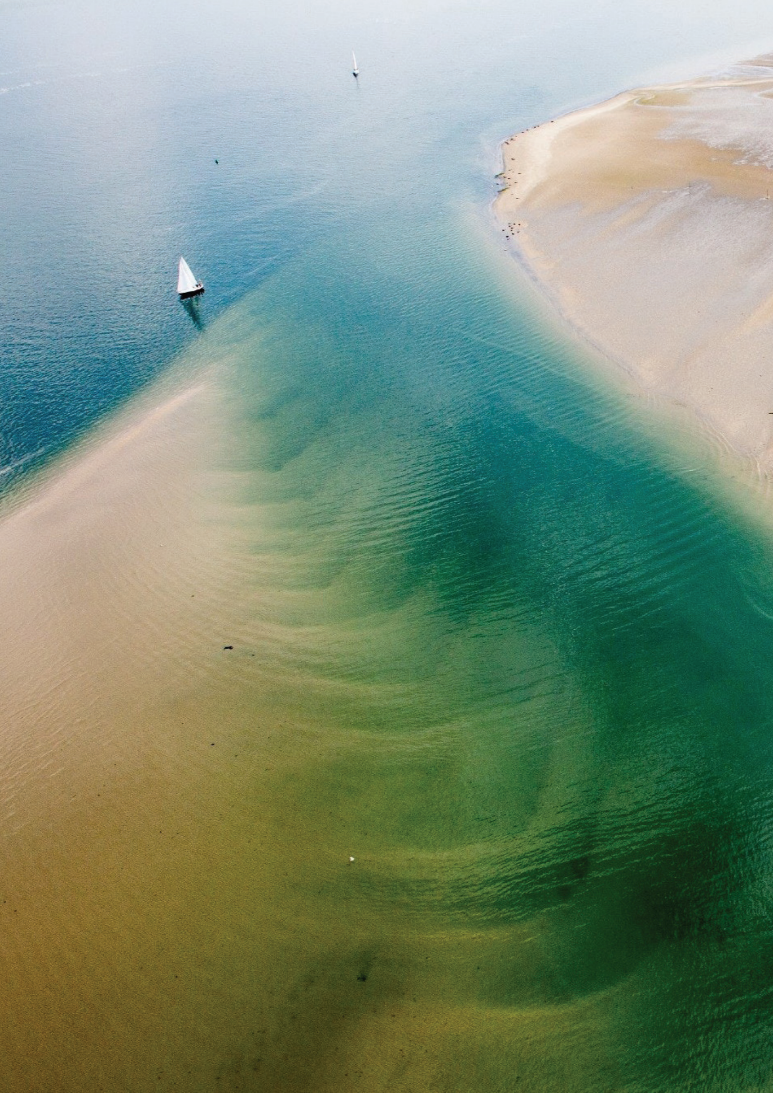
Figure 5.1: Aerial view of the Galgeplaat tidal flat, Oosterschelde. This sandflat is one of the areas losing volume to the sediment starvation that, as Chapter 4 showed, was foreseen and accepted as the price of keeping the Oosterschelde open. Sand nourishment ("zandsuppletie") is now required simply to maintain what the 1976 decision chose to preserve.
