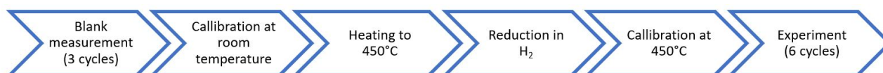
Figure 3.7: A schematic visualization of the protocol to determine the consumption of H_2 .
