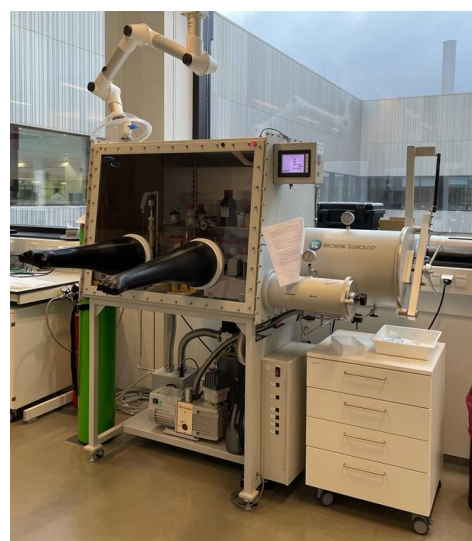
Figure 3.1: Glovebox used for the production of \text{Cu-K}/\gamma\text{-Al}_2\text{O}_3 type 2.
