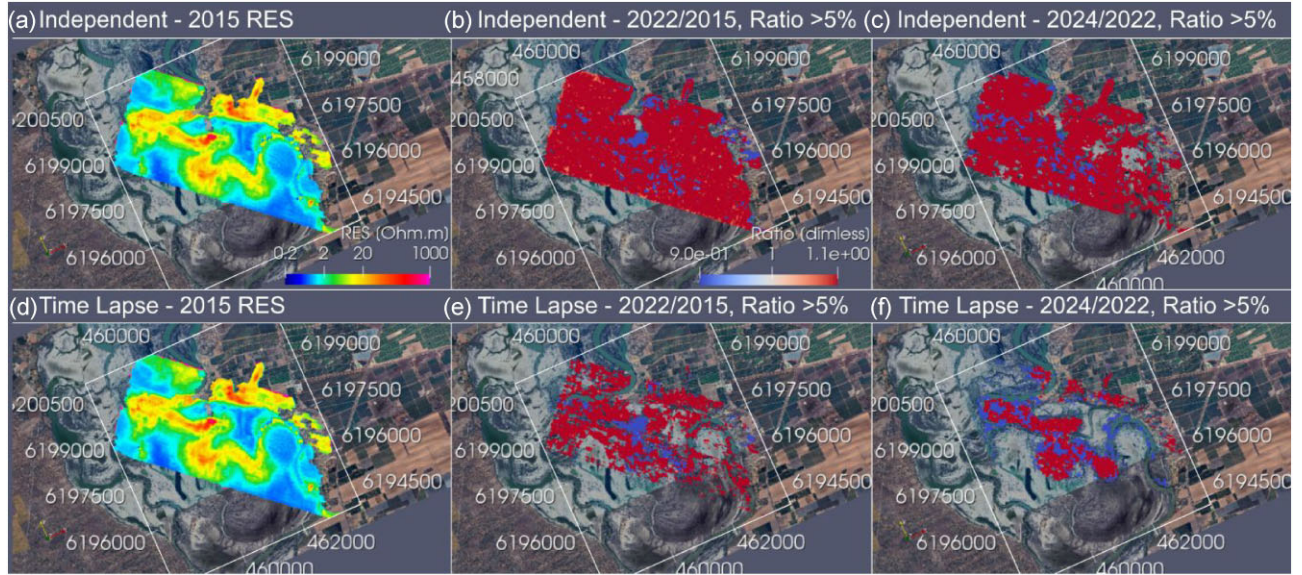
Figure 7. Real-case comparison of independent and time-lapse inversions performed on the Bookpurnong data sets. (a) 2015 resistivity model obtained through independent inversion. (b) Ratio of 2022 to 2015 independent resistivity models. (c) Ratio of 2024 to 2022 independent resistivity models. (d) 2015 resistivity model obtained through time-lapse inversion. (e) Ratio of 2022 to 2015 time-lapse resistivity models. (f) Ratio of 2024 to 2022 time-lapse resistivity models. All ratio model shows differences greater than \pm 5 per cent.
