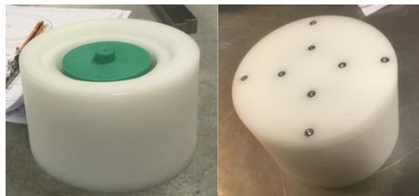
*Figure A1.1 Mold for rubber ring manufacturing*
