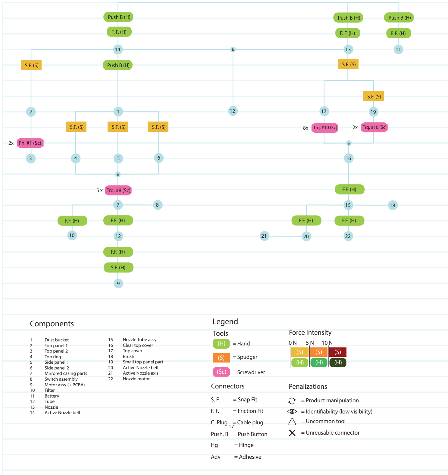
Figure 14 The Disassembly map of the Bosch Unlimited 8 Series
