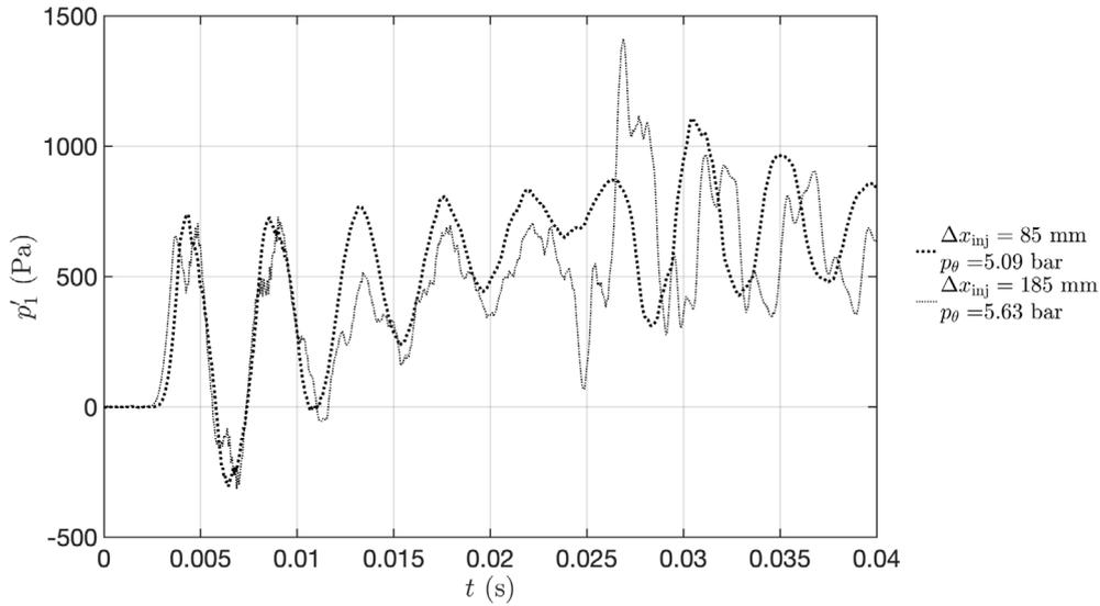
**Fig. 8.** Upstream acoustic pressure signal  $p'_1$  vs. time  $t$ .  $p'_1$  is phase-averaged result of 100 consecutive injection events. Two results are shown, obtained with two different injection port positions,  $\Delta x_{inj}$ , and injection reservoir pressures  $p_\theta$ . The trigger time used to open and close the valve was identical in both measurements:  $\tau_{valve} = 10$  ms.
