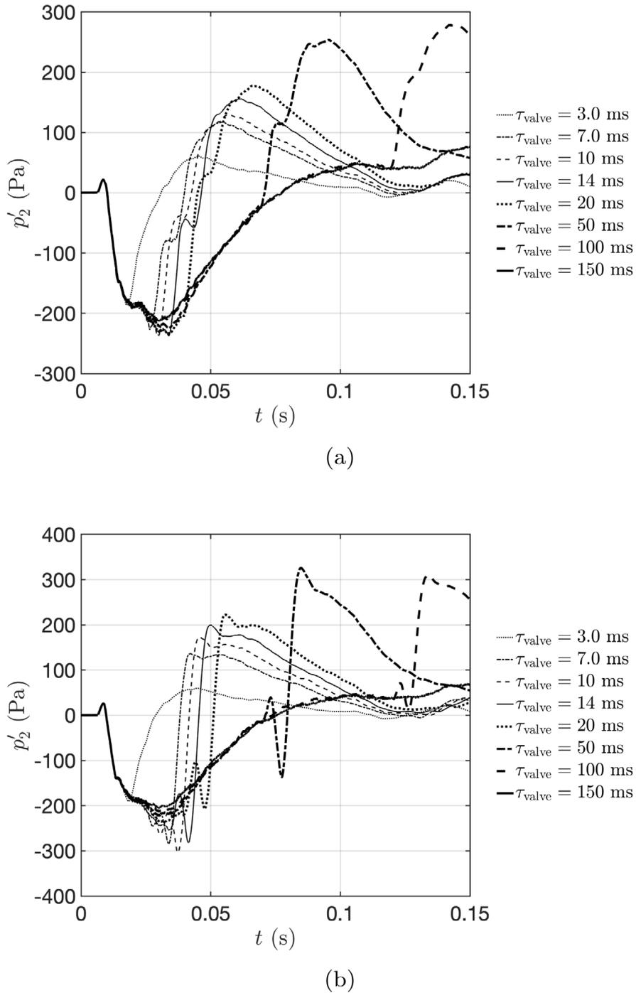
Fig. 9.  $p'_2$  for  $\dot{m}_{\theta,l} = 0.417 \times 10^{-2} \text{ kg s}^{-1}$  into a swirl-free background flow, for varied  $\tau_{\text{valve}}$ . (a)  $\phi_{\theta} = 0^{\circ}$  (b)  $\phi_{\theta} = 10^{\circ}$ .
