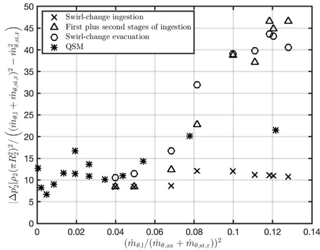
Fig. 15.  $\Delta p'_2$  due to first stage swirl-change ingestion (crosses), first plus second stages of ingestion (triangles), swirl-change evacuation (circles). Empirical data are compared to the QSM predictions (stars).
