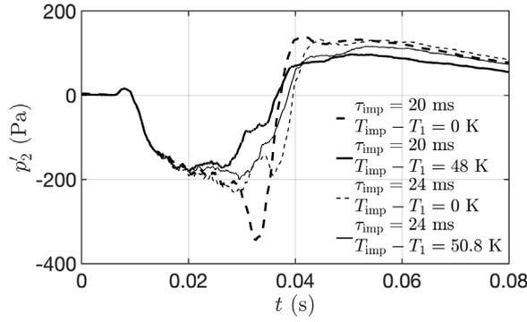
Fig. 16. Comparison of the downstream acoustic response  $p'_2$  to tangential-injection for  $p_{imp} = 6.2$  bar,  $\tau_{imp} = 20$  ms (thick lines) and  $\tau_{imp} = 24$  ms (thin lines). The dashed and the solid lines correspond to unheated- and heated-air tangential-injection experiments, respectively.
