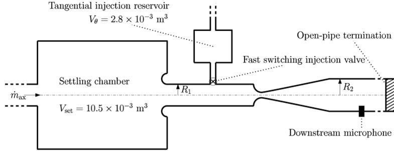
Fig. 4. Sketch of the entropy-swirl-nozzle interaction experimental setup.
