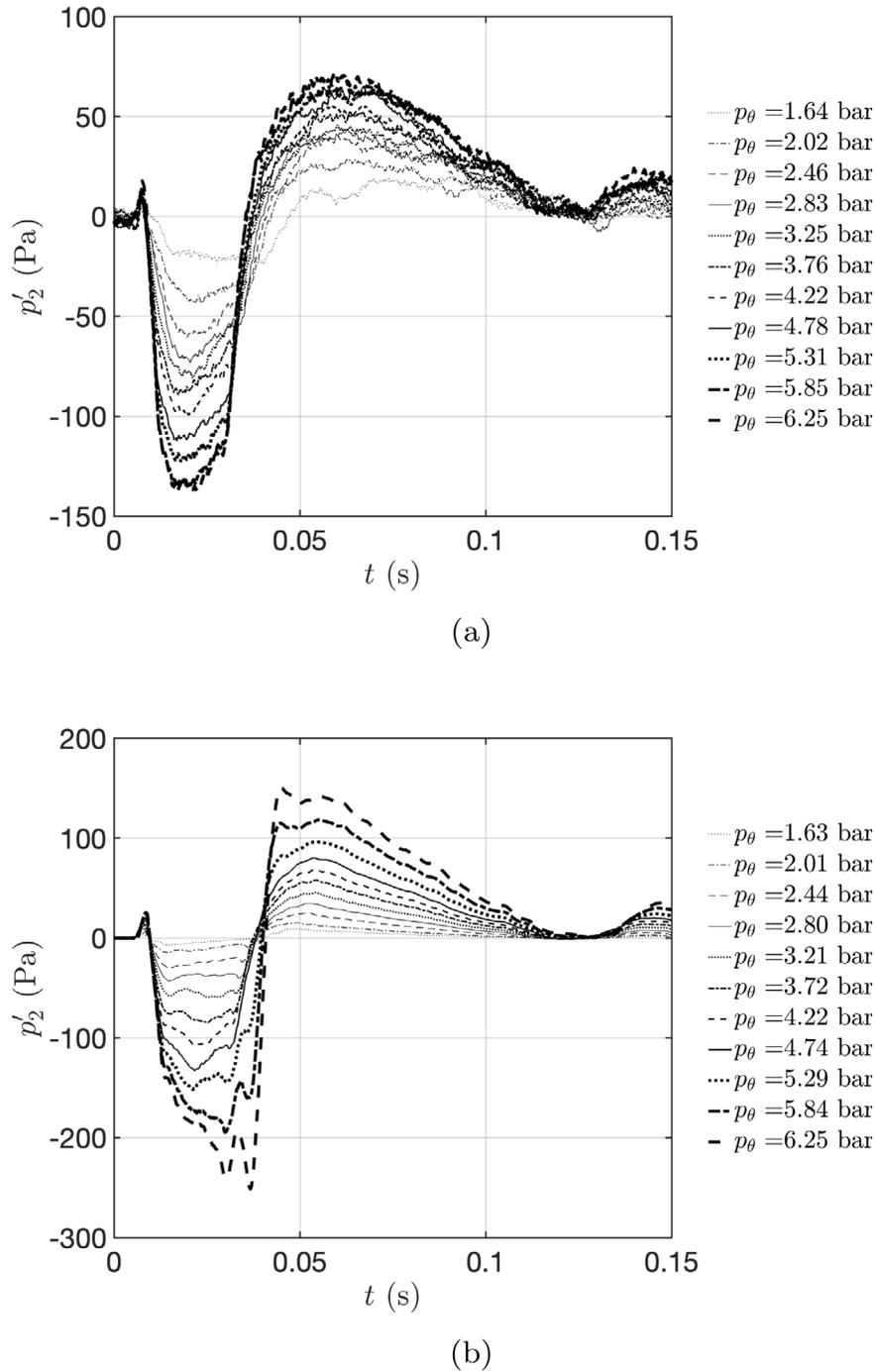
**Fig. 12.** Comparison of  $p'_2$  in presence (a) and absence (b) of a high-intensity background swirl. In both cases  $\tau_{\text{valve}} = 10$  ms. (a)  $\dot{m}_{\theta, \text{st}, r} = 0.472 \times 10^{-2}$  kg s $^{-1}$  and  $\dot{m}_{\text{ax}} = 0.722 \times 10^{-2}$  kg s $^{-1}$  (b)  $\dot{m}_{\theta, \text{st}, r} = 0$  and  $\dot{m}_{\text{ax}} = 1.194 \times 10^{-2}$  kg s $^{-1}$ .
