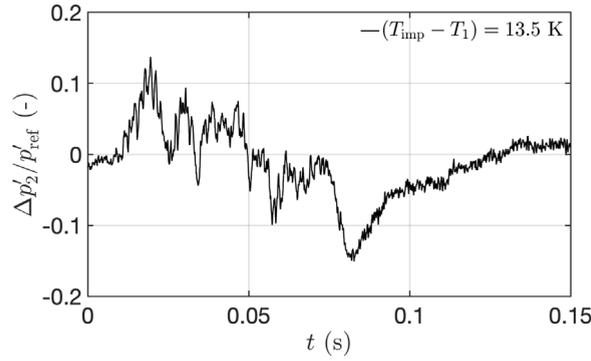
Fig. 17. Dimensionless difference  $\Delta p'_2/p'_{\text{ref}}$  between heated and unheated impulsive-injection signals due to radial injection for  $T_{\text{imp}} - T_1 = 13.5$  K,  $p_{\text{imp}} = 5.2$  bar and  $\tau_{\text{imp}} \approx 62$  ms.
