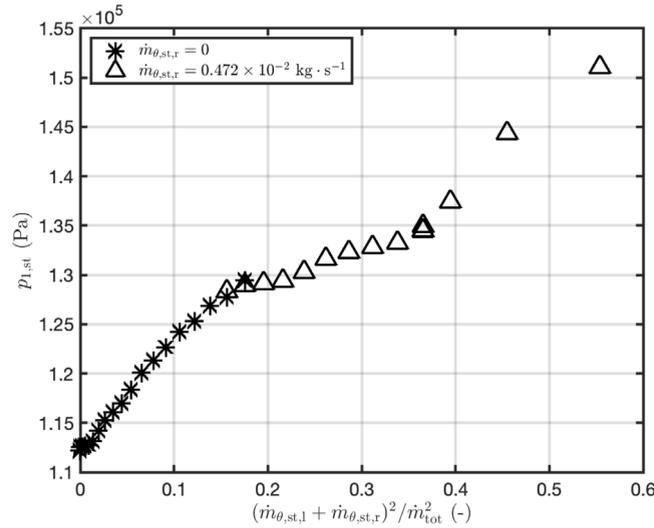
Fig. 5. Influence of  $(\dot{m}_{\theta, \text{st},1} + \dot{m}_{\theta, \text{st},r})^2 / \dot{m}_{\text{tot}}^2$  on  $p_{1, \text{st}}$  where  $\dot{m}_{\text{tot}} = 1.194 \times 10^{-2} \text{ kg s}^{-1}$ .
