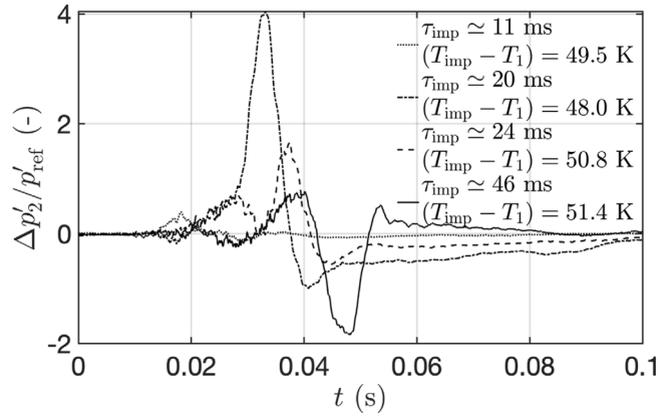
Fig. 18. Dimensionless difference  $\Delta p'_2/p'_{ref}$  between heated and unheated impulsive-injection signals due to tangential injection. Dotted line  $\tau_{imp} = 12$  ms, dotted-dashed line  $\tau_{imp} = 20$  ms, dashed  $\tau_{imp} = 24$  ms, solid line  $\tau_{imp} = 46$  ms.
