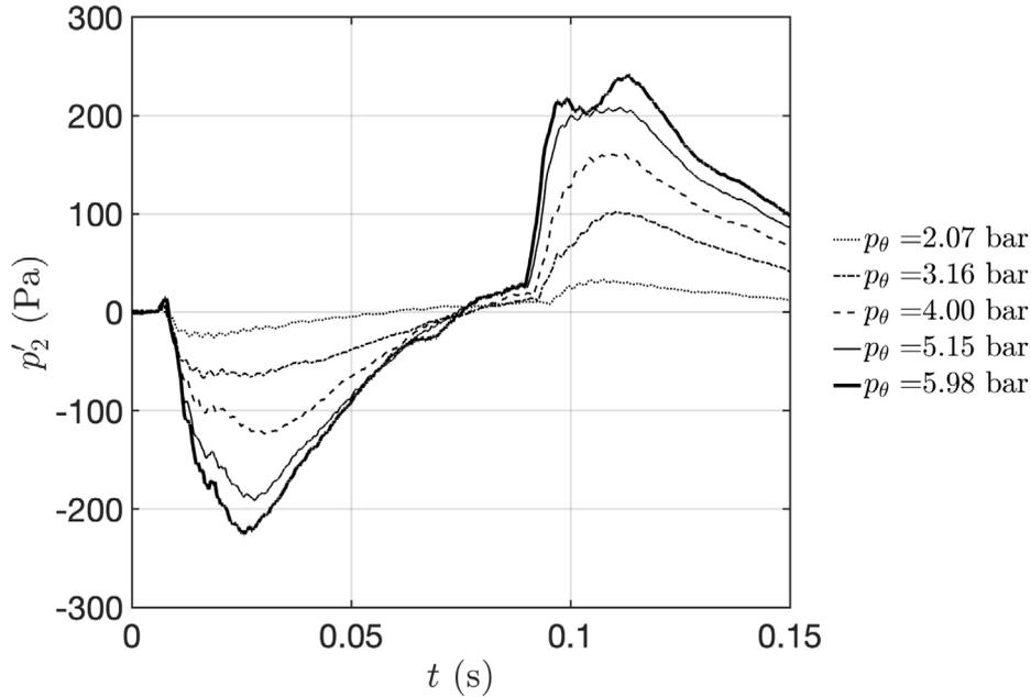
Fig. 11.  $p'_2$  due to the perturbation of low-intensity steady-background swirl, for  $\dot{m}_{ax} = 1.00 \times 10^{-2}$  kg s $^{-1}$ ,  $\dot{m}_{\theta, st, r} = 1.94 \times 10^{-3}$  kg s $^{-1}$  and  $\tau_{\text{valve}} = 70$  ms.
