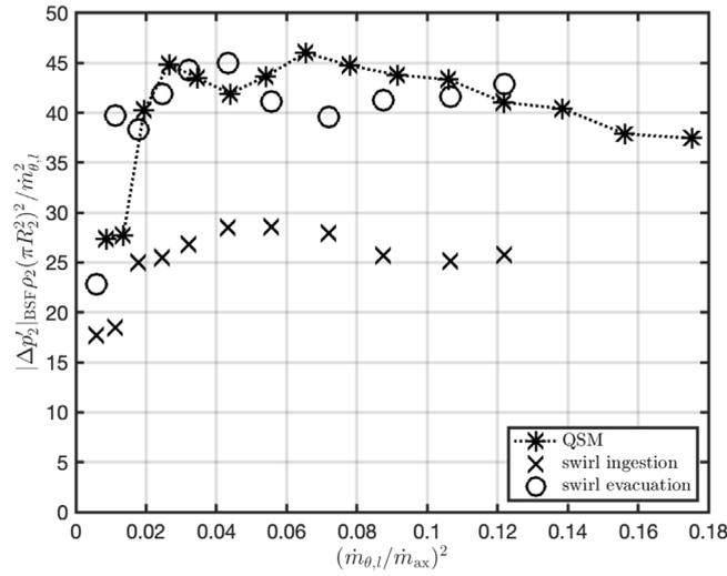
Fig. 10. Dimensionless  $\Delta p'_2$  due to either the ingestion (crosses) or evacuation (circles) of swirl compared to QSM prediction (dotted-line connected stars). Results obtained with  $\tau_{\text{valve}} = 50$  ms.
