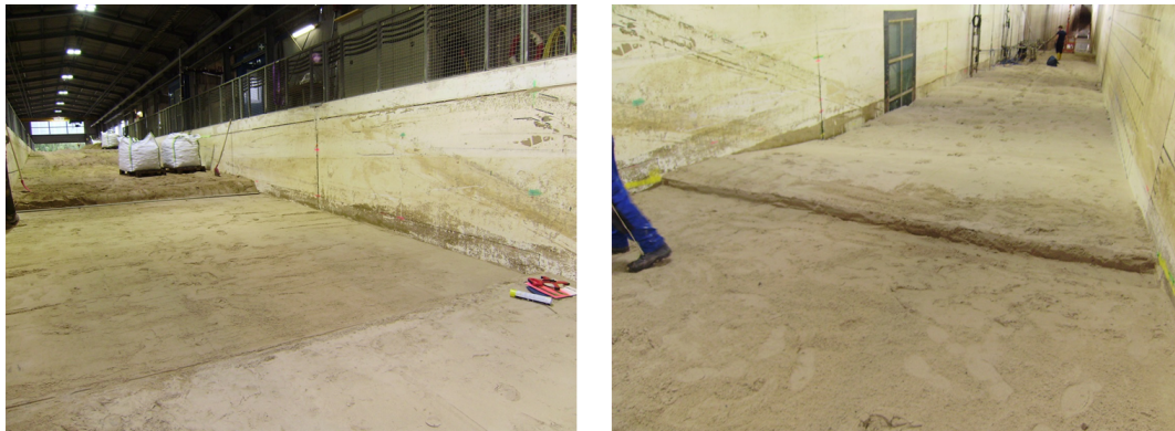
Figure B.6: Pictures of sand bed before placement of gravel revetment - Pictures by Paul Maxime Bayle
