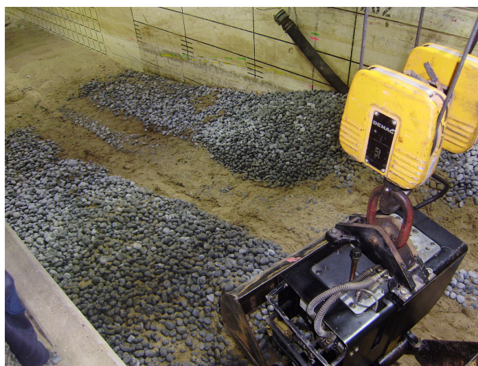
Figure B.7: Picture of bottom of revetment with the gravel stones removed - Picture by Paul Maxime Bayle
