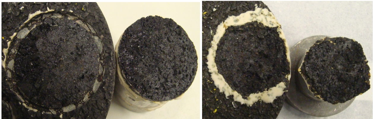
Figure 5 Failure surfaces at the interface
