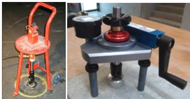
Figure 1 Sample pull test setups that can be used in the fields
