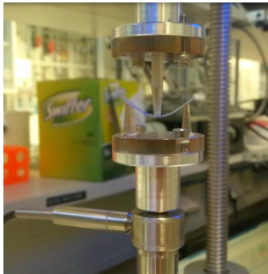
Figure 13 3-point bending test measurement setup
