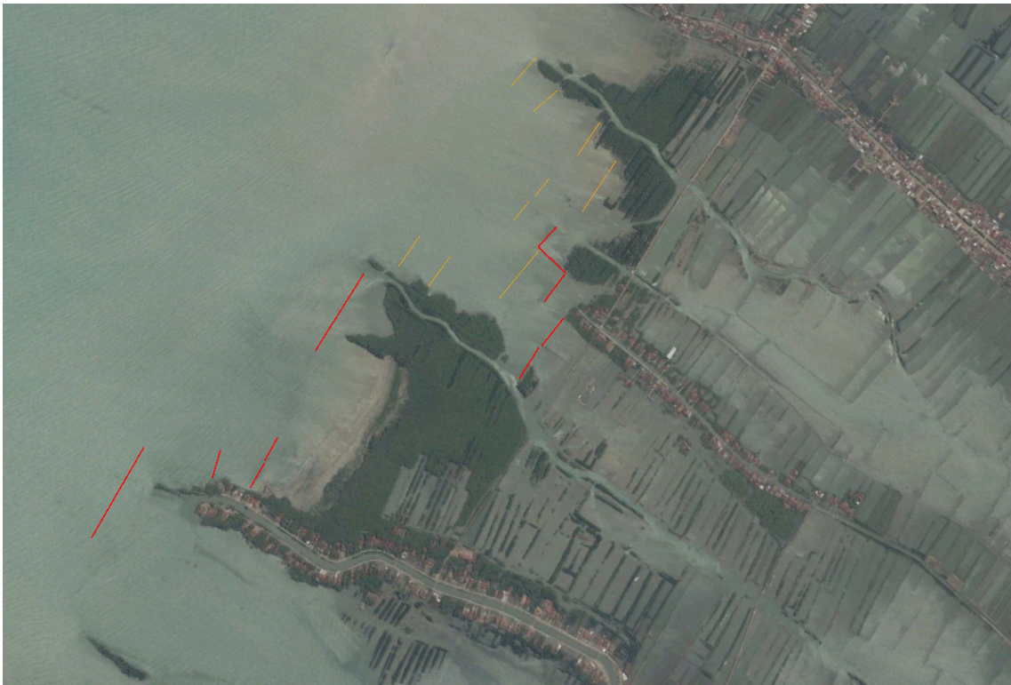
Figure 4.4: An overview of constructed dams for the pilot study by Ecoshape (shown in red) and MMAF (orange)
