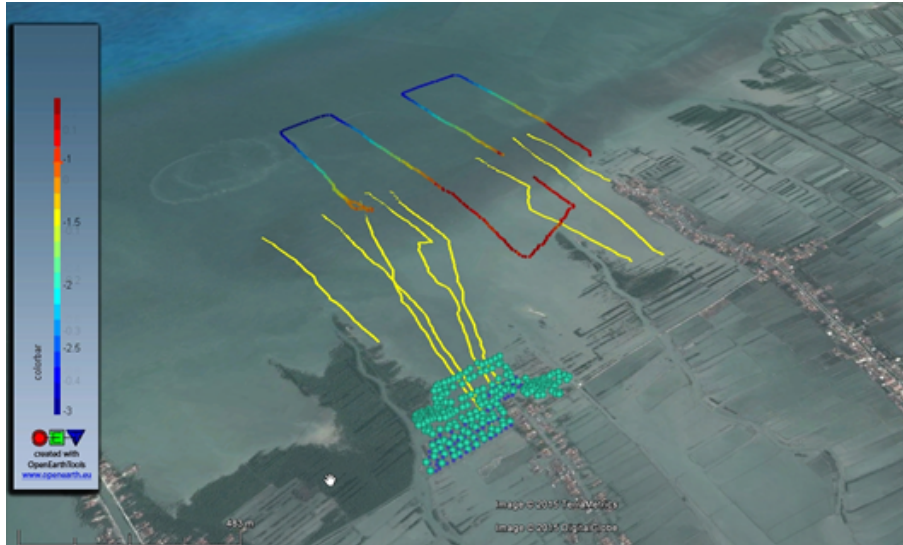
Figure F.1: Locations of depth measurements performed by Stefan Verschure
