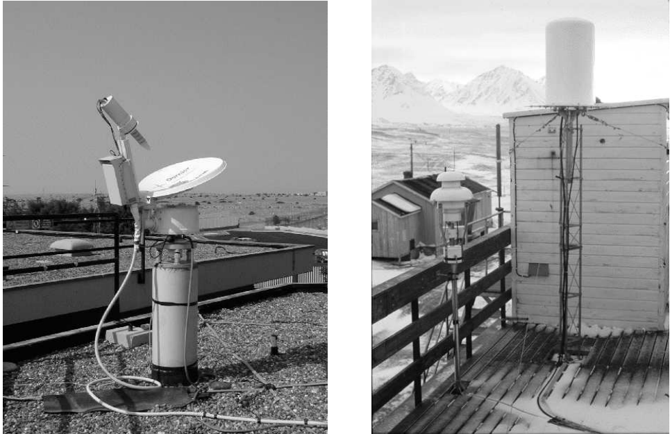
Figure 3.5 Left: PRARE transponder at Matera, Italy. Right: DORIS beacon at Ny Ålesund, Norway.
