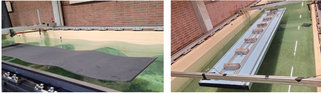
Fig. 4. Floating structures moored in the towing tank facility, (left) flexible and (right) rigid structure.
