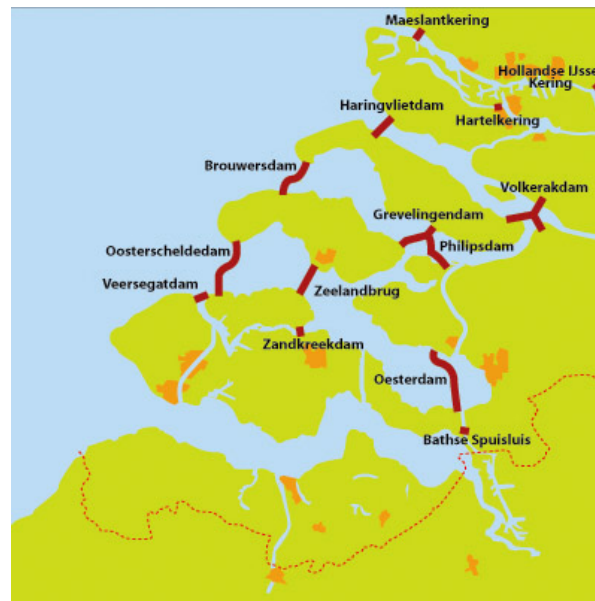
Figure 2.2: Overview of the different storm surge barriers and dams that were constructed as part of the Deltaworks after the 1953 North Sea Flood.
