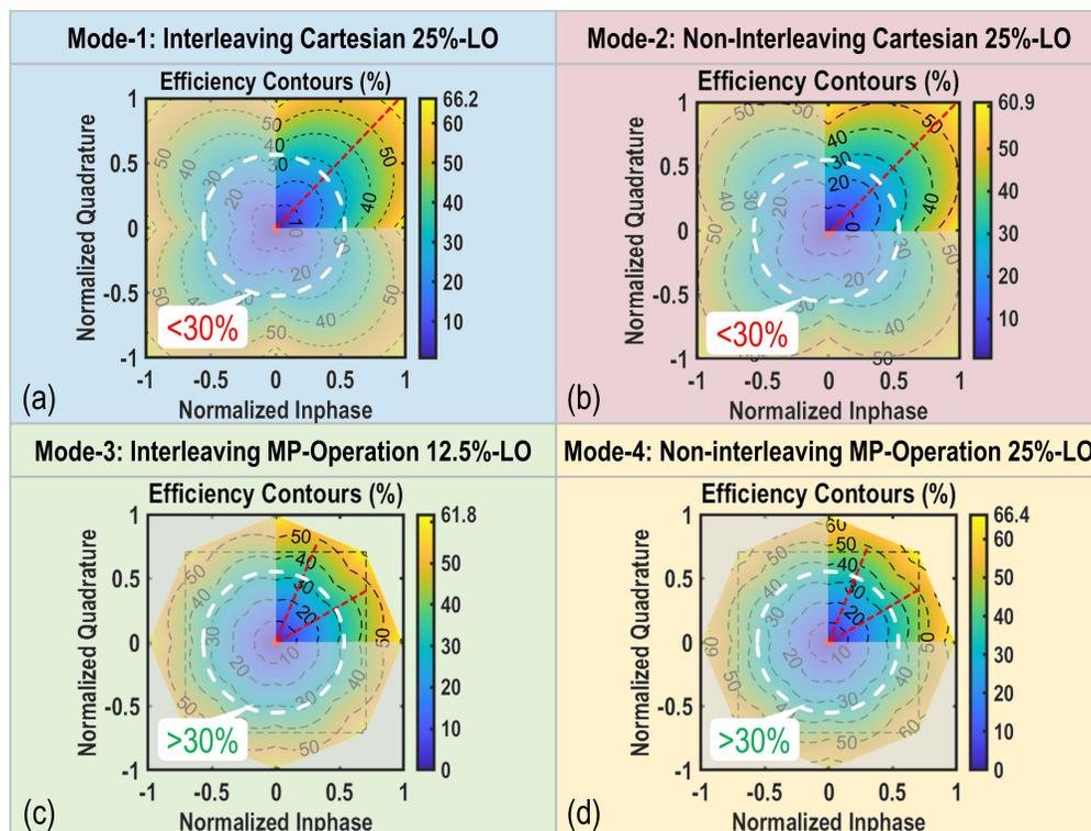
Figure 3.25: The measured drain efficiency contours of the 400-point static points using 20 samples for each  $I/Q$  symbol in the first  $I/Q$  quadrant at 2.4GHz extracted for the four-quadrant plane for different operational modes.
