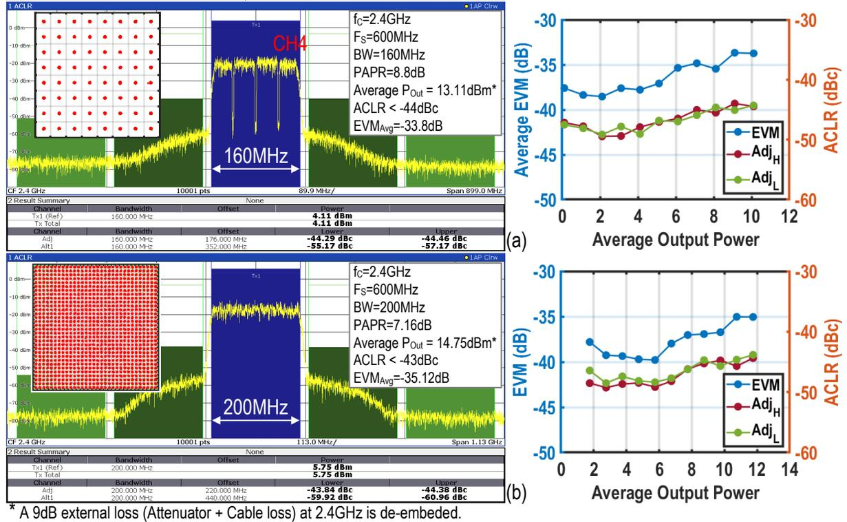
Figure 4.9: Measured results of (a) 4-channel $\times$ 40MHz 64-QAM signal, and (b) single-channel 200MHz 1024-QAM signal at 2.4GHz.
