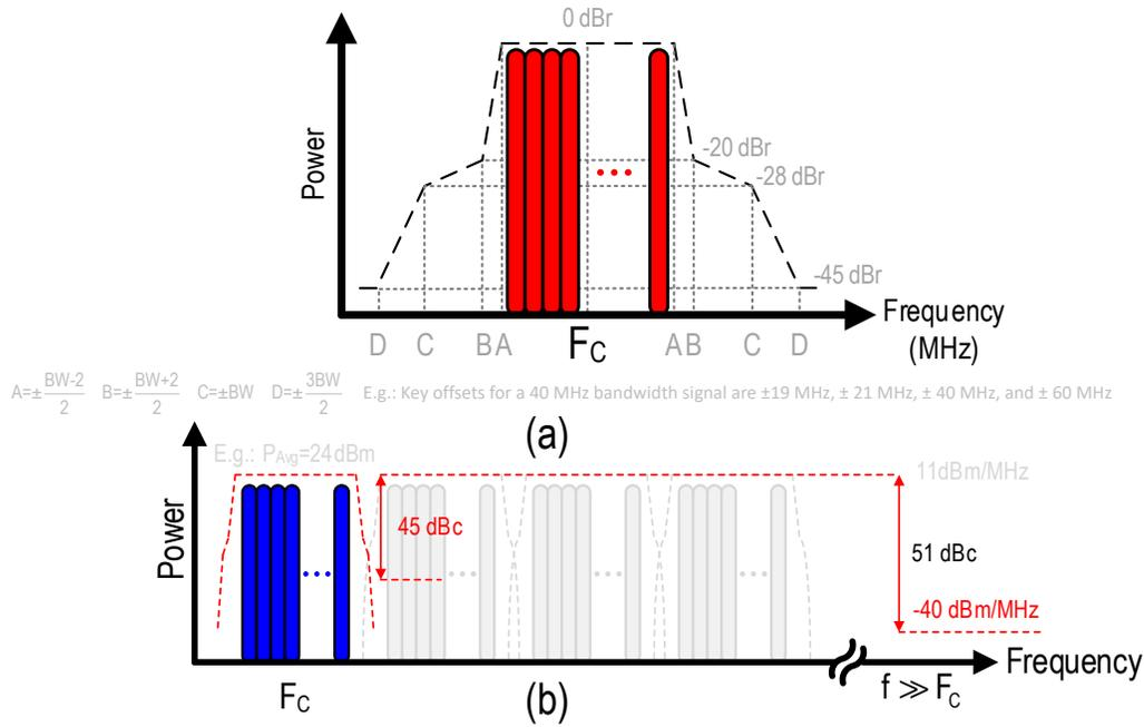
Figure 1.8: (a) Spectral mask. (b) Spurious emission.
