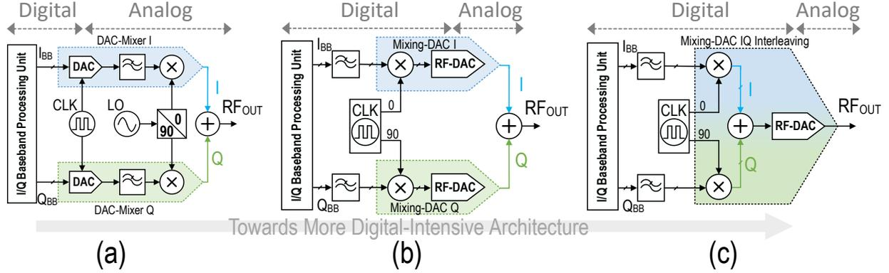
Figure 2.8: The evolution of digital-intensive Cartesian transmitters. (a) Analog Cartesian, (b) mixing of the data and LO in the digital domain, and (c) digital  $I/Q$  combination.
