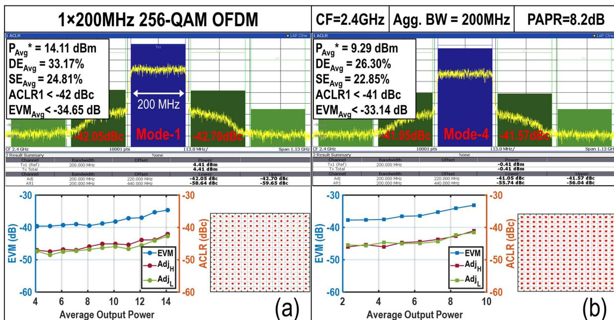
Figure 3.29: Measured spectrum of single-channel  $\times 200\text{MHz}$  256-QAM OFDM signal, its constellation diagram, and ACLR and average EVM performances versus average output power for Mode-1/-4 operation.
