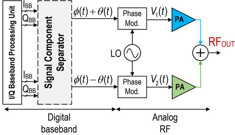
Figure 2.14: Outphasing or LINC efficiency enhancement architecture.
