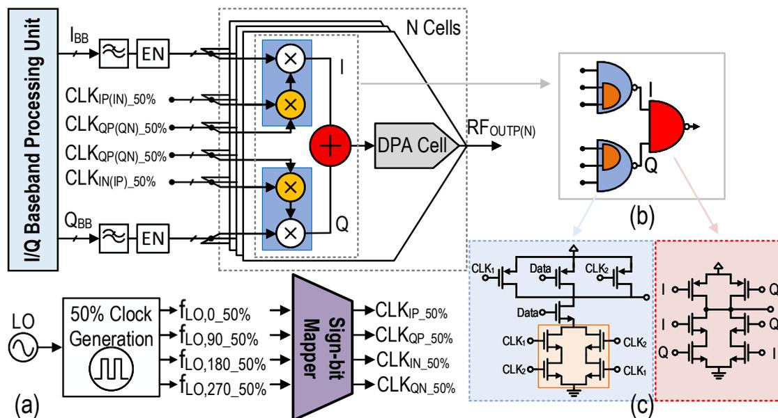
Figure 5.7: (a) Schematic diagram of the local 25%-LO clock generation,  $I/Q$  up-conversion, and interleaving. (b) NAND gate-based logical implementation circuitry. (c) 2-/3-input symmetrical NAND logic gates.
