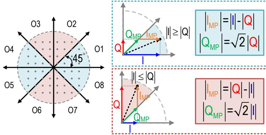
Figure 3.4: Multi-phase (eight-phase) operation baseband data mapping depending on the corresponding octant.
