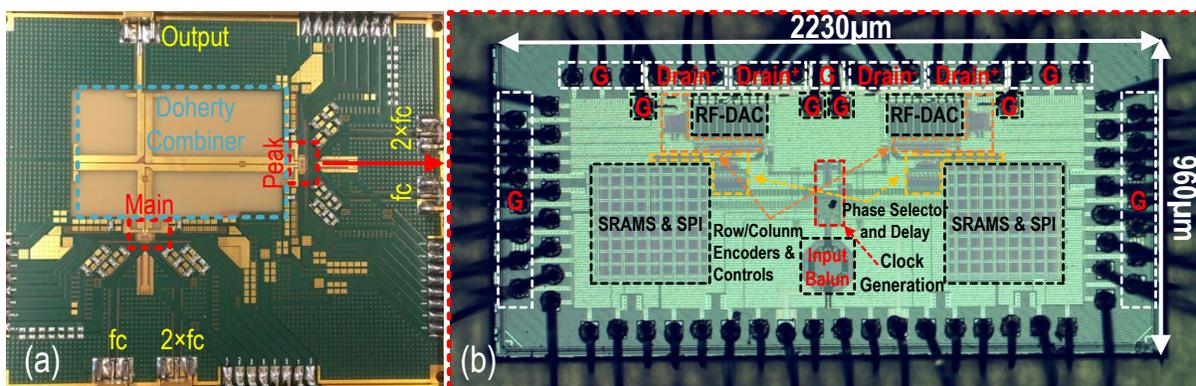
Figure 4.4: (a) Fabricated PCB (b) Die micrograph.
