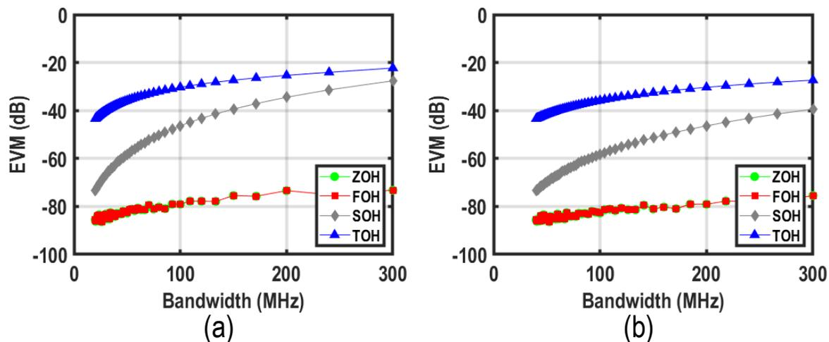
Figure A.6: EVM performance of ZOH, FOH, SOH, and TOH interpolation filters applied to a pulse-shaped 256-QAM  $I/Q$  baseband depending on signal bandwidth while their corresponding  $L_{SRC}$  is (a) 8, and (b) 4.
