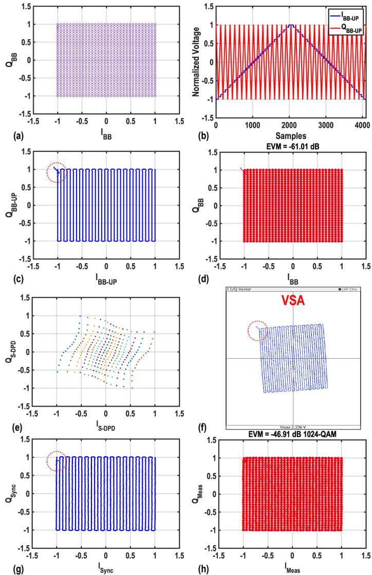
Figure 6.6: DPD measurements: (a) 1024-QAM constellation diagram ( $I_{BB}/Q_{BB}$ ); (b) Trajectories of their related time domain waveforms; (c),(d)  $I_{BB-UP}/Q_{BB-UP}$  trajectories; (e) predistorted  $I_{DPD}/Q_{DPD}$  trajectories; (f) measured  $I_{DW}/Q_{DW}$  trajectories; (g) measured  $I_{Sync}/Q_{Sync}$  trajectories (h) measured 1024-point constellation.
