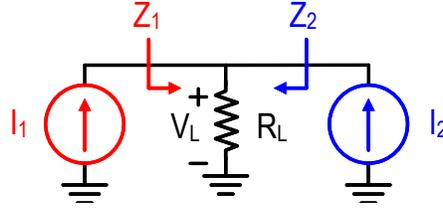
Figure 2.12: An illustration of the active load-pull concept.
