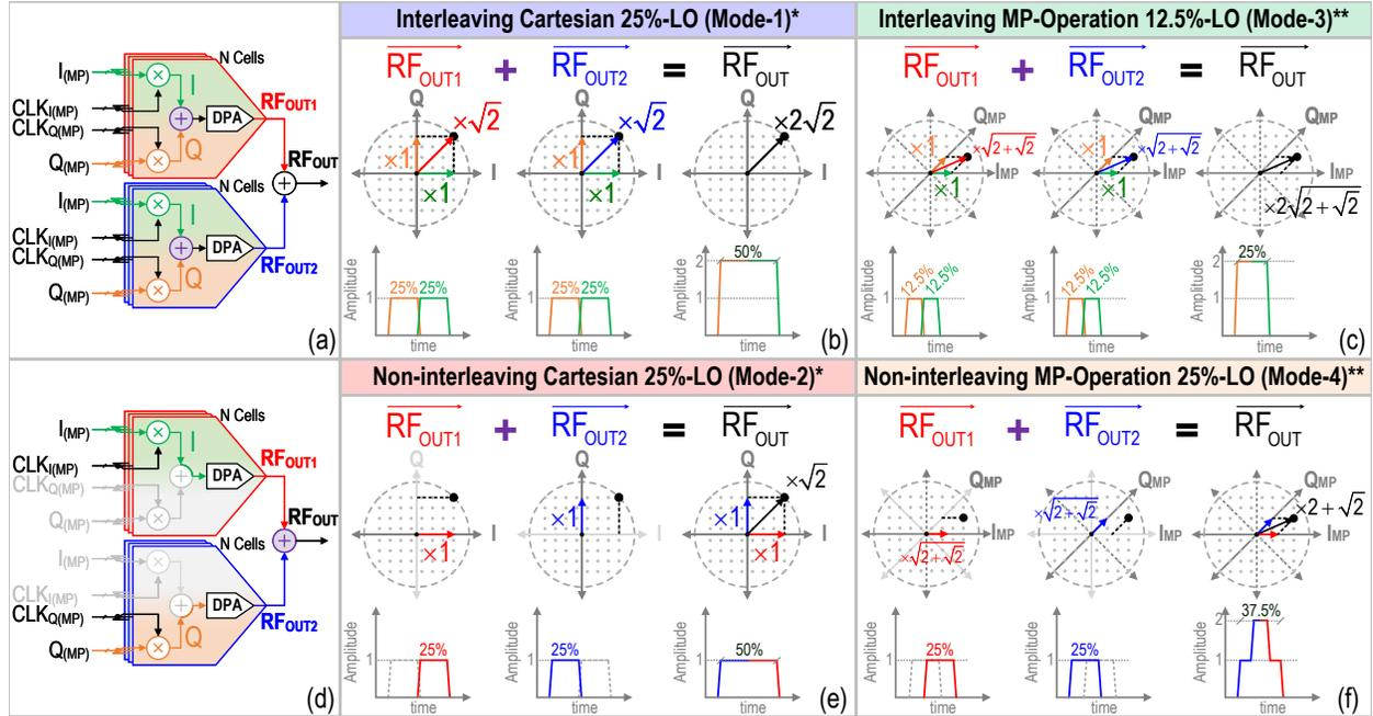
Figure 3.8: The overall operating modes of the proposed DTX. (a) Interleaving and (d) non-interleaving configurations. In the (b) Mode-1 and (e) Mode-2 cases the  $I/Q$  vectors are normalized to  $\frac{D}{\pi}$ . In the (c) Mode-3 and (e) Mode-4 scenarios the  $I_{MP}/Q_{MP}$  vectors are normalized to  $\frac{D \sin(\frac{\pi}{8})}{\pi}$ .
