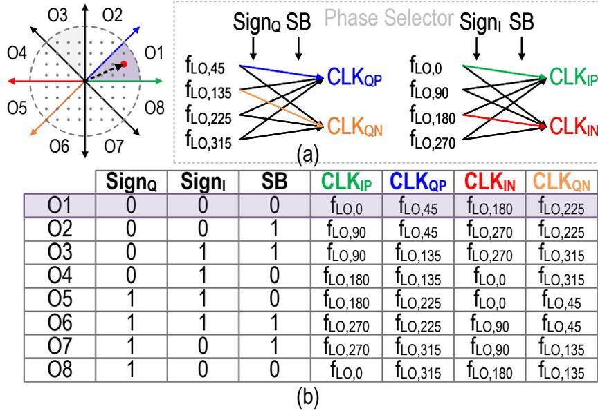
Figure 3.5: (a) Multi-phase (eight-phase) DTX phase selector (sign-bit) operation utilizing Sign<sub>I</sub>, Sign<sub>Q</sub> and Sector-Bit (SB). (c) Associated swapped complementary clock pairs based on the operating octant.
