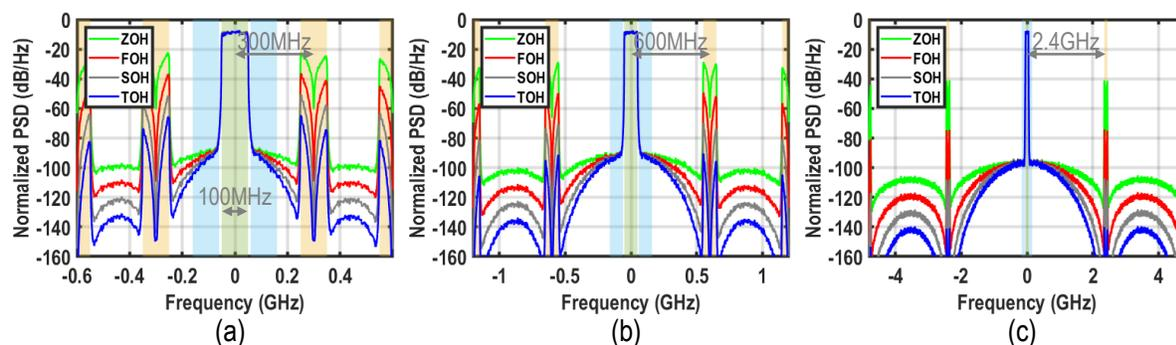
Figure A.4: Power spectral density of ZOH, FOH, SOH, and TOH interpolation filters applied to a pulse-shaped 256-QAM  $I/Q$  baseband signal with 100MHz bandwidth while their corresponding  $L_{SRC}$  is (a) 8, (b) 4, and (c) 1, respectively.
