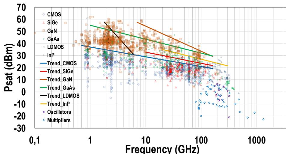
Figure 1.4:  $P_{\text{Sat}}$  comparison between different technologies over frequency [5].
