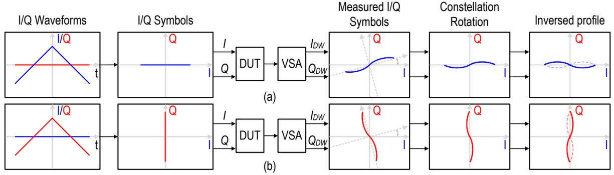
Figure 6.3: Practical,  $V_I(I_{BB-UP}, 0)$  and  $V_Q(0, Q_{BB-UP})$  extraction: (a) in-phase (I) path ramp function while the quadrature (Q) path is zero; (b) quadrature (Q) path ramp function while the in-phase (I) path is zero.
