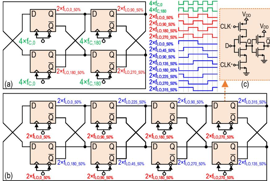
Figure 3.17: (a) Four-phase and (b) eight-phase divide-by-2 circuits with corresponding waveforms. (c) C<sup>2</sup>MOS latch with swapped data/clock inputs.
