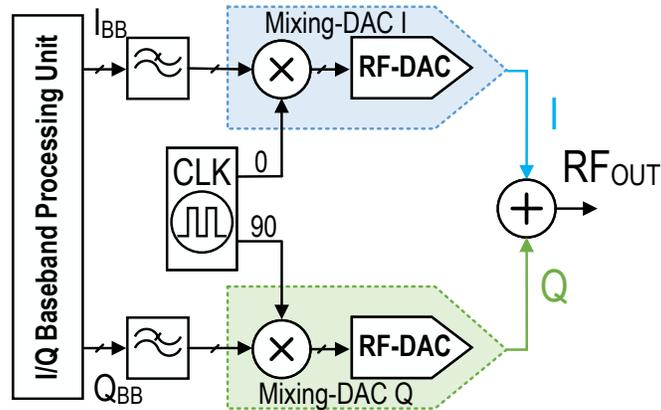
Figure 2.7: Block diagram of a Cartesian DTX.
