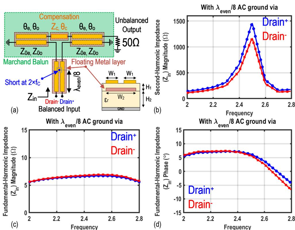
Figure 3.15: (a) Compensated Marchand balun with re-entrant coupled lines and AC grounding at  $\lambda/8$  for the second harmonic control, using a via from the floating metal layer to the ground plane. (b) EM simulation of Fundamental and Second-harmonic impedance class-E load network.
