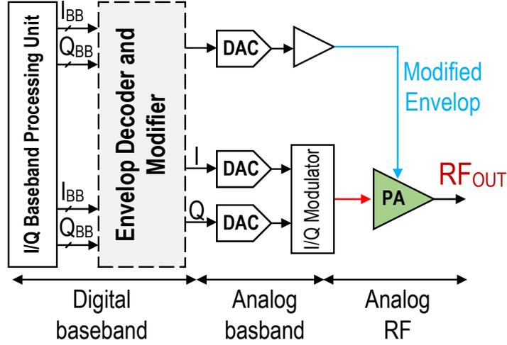
Figure 2.15: Envelope Tracking (ET) efficiency enhancement architecture.
