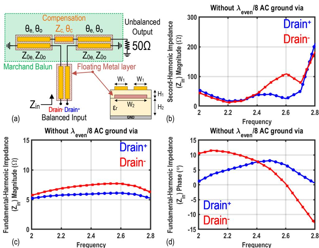
Figure 3.14: (a) Compensated Marchand balun with re-entrant coupled lines and without AC grounding at  $\lambda/8$  for the second harmonic control (b) EM simulation of Fundamental and Second-harmonic impedance class-E load network with a floating island.
