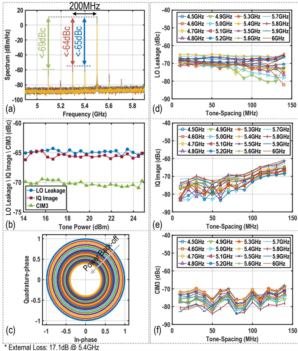
Figure 5.22: Measured (a) output spectrum of a single-tone test with 200MHz tone-spacing at 5.4GHz versus power back-off, (b) its corresponding LO leakage,  $I/Q$  image, and C-IMD3/ $H_{3BB}$ , and (c)  $I/Q$  trajectory. (d)-(f) Measured single-sideband performance over frequency band vs. tone-spacing.
