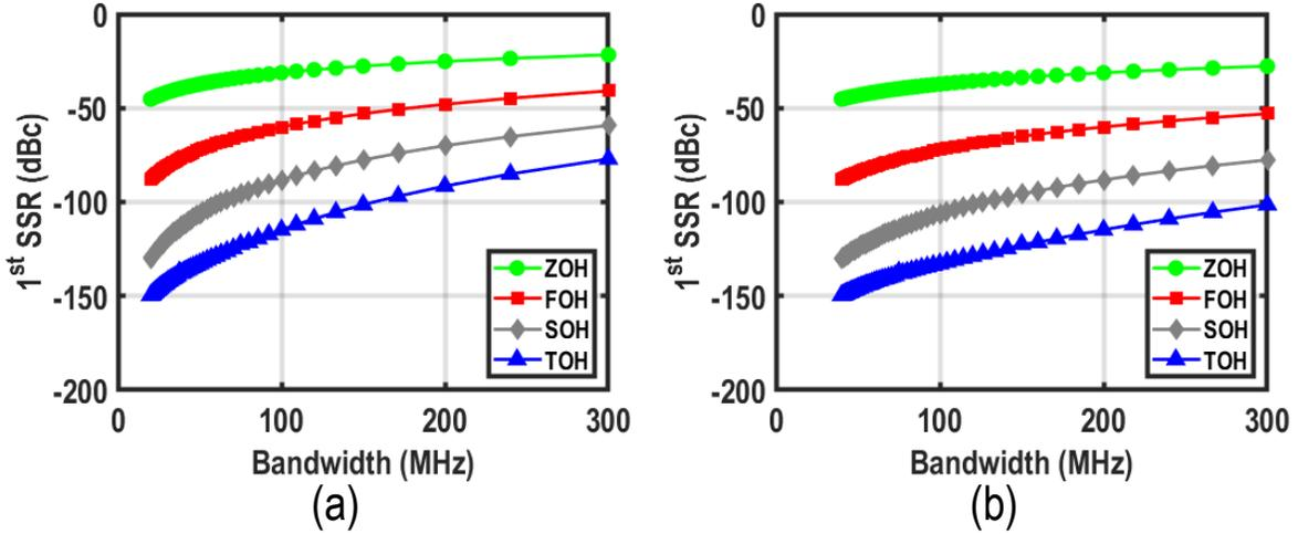
Figure A.5: First sampling spectral replica suppression performance of ZOH, FOH, SOH, and TOH interpolation filters applied to a pulse-shaped 256-QAM  $I/Q$  baseband depending on signal bandwidth while their corresponding  $L_{SRC}$  is (a) 8, and (b) 4.
