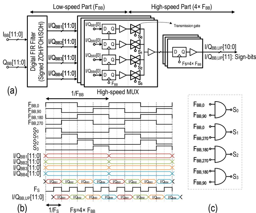
Figure 5.17: Interpolation filter and its high-speed MUX: (a) Detailed implementation. (b) Corresponding waveforms. (c) Generating MUX selection signals from different phases of the  $F_{BB}$  clock [59].
