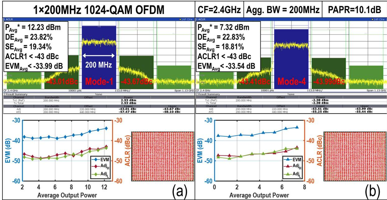
Figure 3.30: Measured spectrum of single-channel $\times$ 200MHz 1024-QAM OFDM signal, its constellation diagram, and ACLR and average EVM performances versus average output power for Mode-1/-4 operation.
