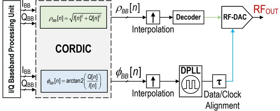
Figure 2.10: Block diagram of a polar DTX.
