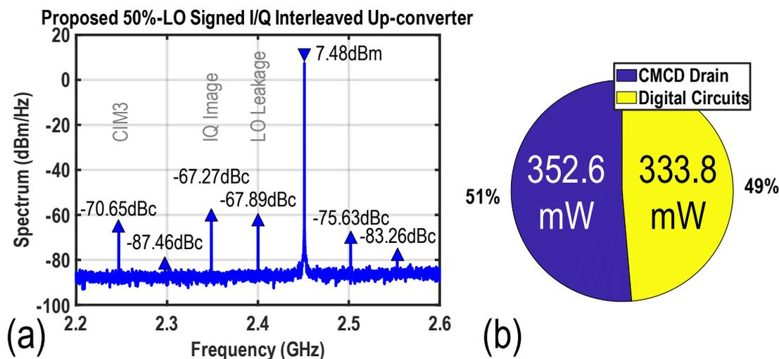
Figure 5.8: (a) Single-sideband spectrum with 100MHz tone-spacing at 2.4GHz employing the proposed 50%-LO signed  $I/Q$  interleaving up-converter. (b) Power consumption breakdown.
