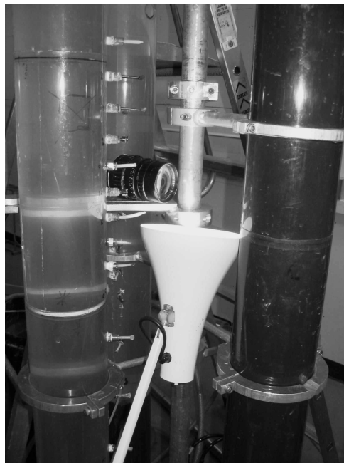
Figure 4.6. Set-up of light and camera for the PTV and PIV measurements.
