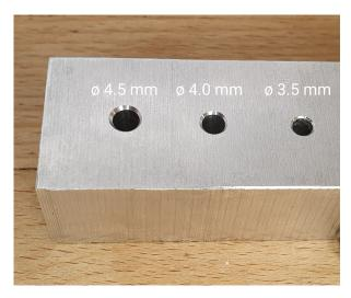
Figure 3.3: Aluminum block featuring three holes of varying diameters (3.5 mm, 4.0 mm, and 4.5 mm). Used to assess the feasibility of inserting the different configurations of silicone rings.
