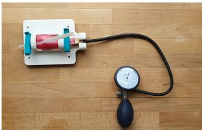
Figure M.4: The umbilical vessels are secured with the sealing clips, ensuring the umbilical cord is centered, and the pressure is set at 10 mmHg.
