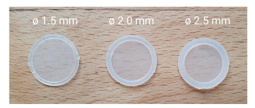
Figure 3.4: Three configurations of the silicone ring with membrane produced during the first prototyping round with varying cord sizes (1.5 mm, 2.0 mm, and 2.5 mm). Notably, the 1.5 mm ring displays visible air bubbles as well as a remnant of the cut rod originating from the injection hole. Additionally, the 2.5 mm ring exhibits slight traces of silicone on its outer surface.
