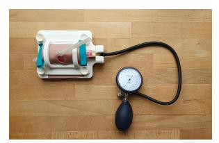
Figure M.5: The top and base are fastened together with the abdominal wall in between, and the pressure is set to 20 mmHg.
