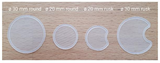
Figure 3.7: The four configurations of the silicone ring with membrane produced during the final prototyping round with varying shapes (round or rusk) and varying diameters (20 mm or 30 mm). Notably, the membranes exhibit an unintentional striped pattern.
