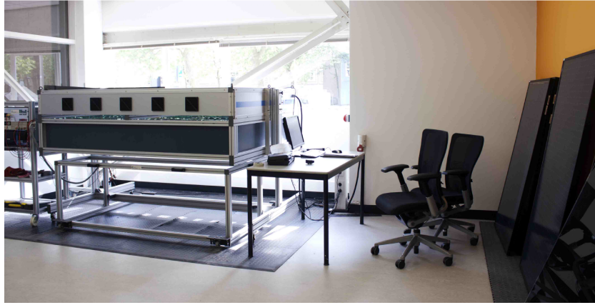
Figure 4.1. The Large Area Solar Simulator (LASS) used in the PV Lab to perform I-V curve measurements.
