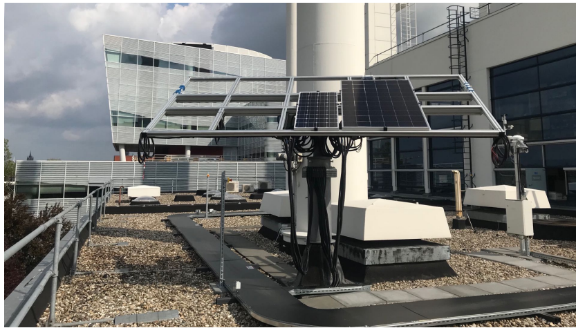
Figure 4.2. The studied solar module in the PVMD monitoring system (the left one on the rack).
