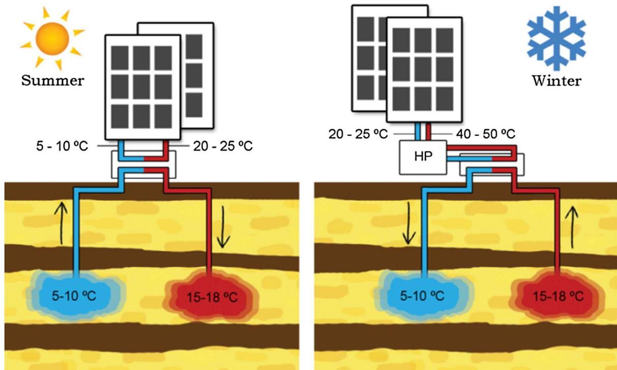
**Figure 13.** Schematic visual of an ATES system with doublet [Z3]
