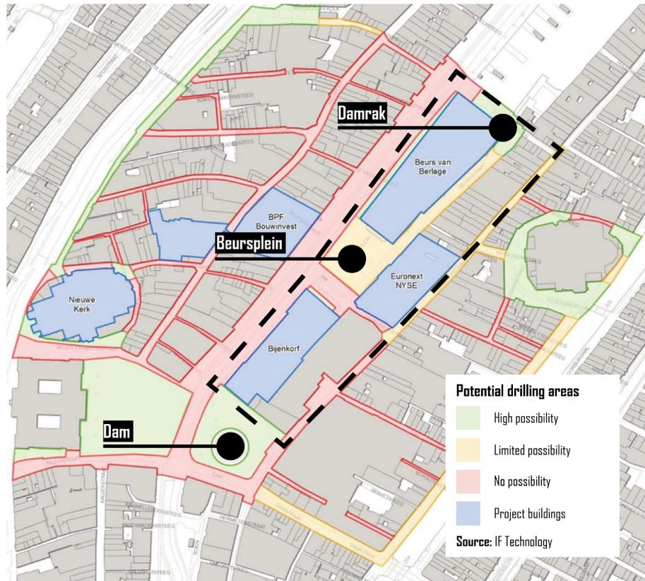
Figure 16. Potential drilling areas for thermal storage systems [71]
