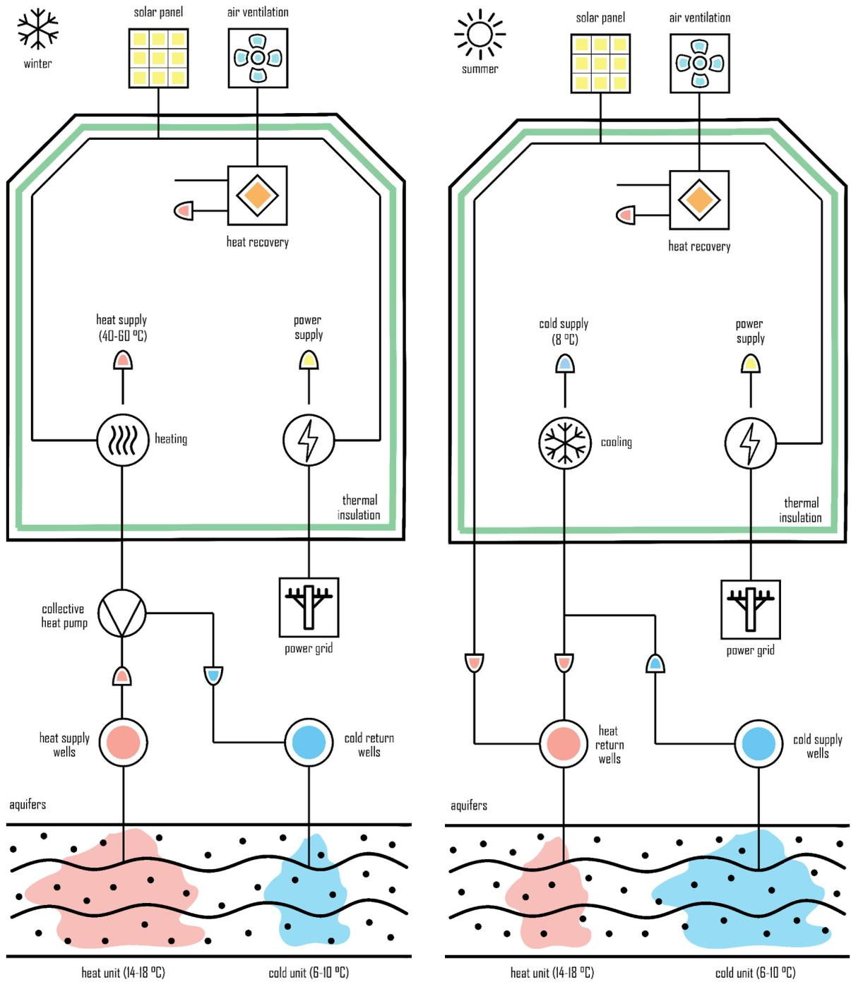
Figure 21 & 22. Schematic diagrams of Option C for heating and cooling
