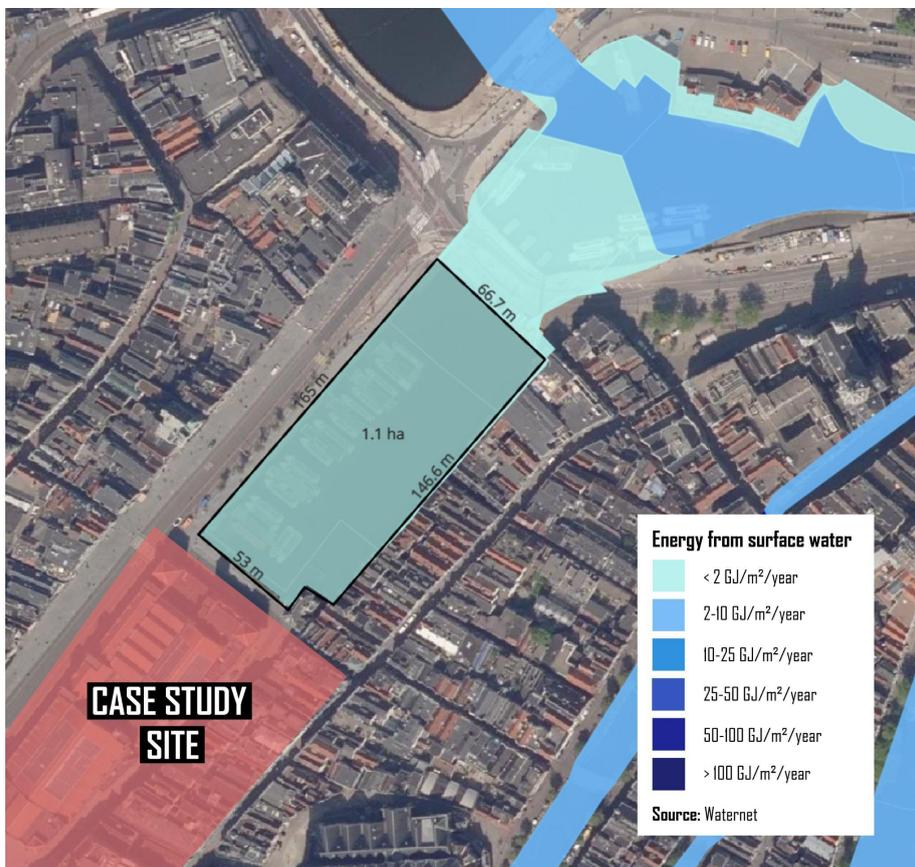
Figure 18. Energy potential from surface water [82]
