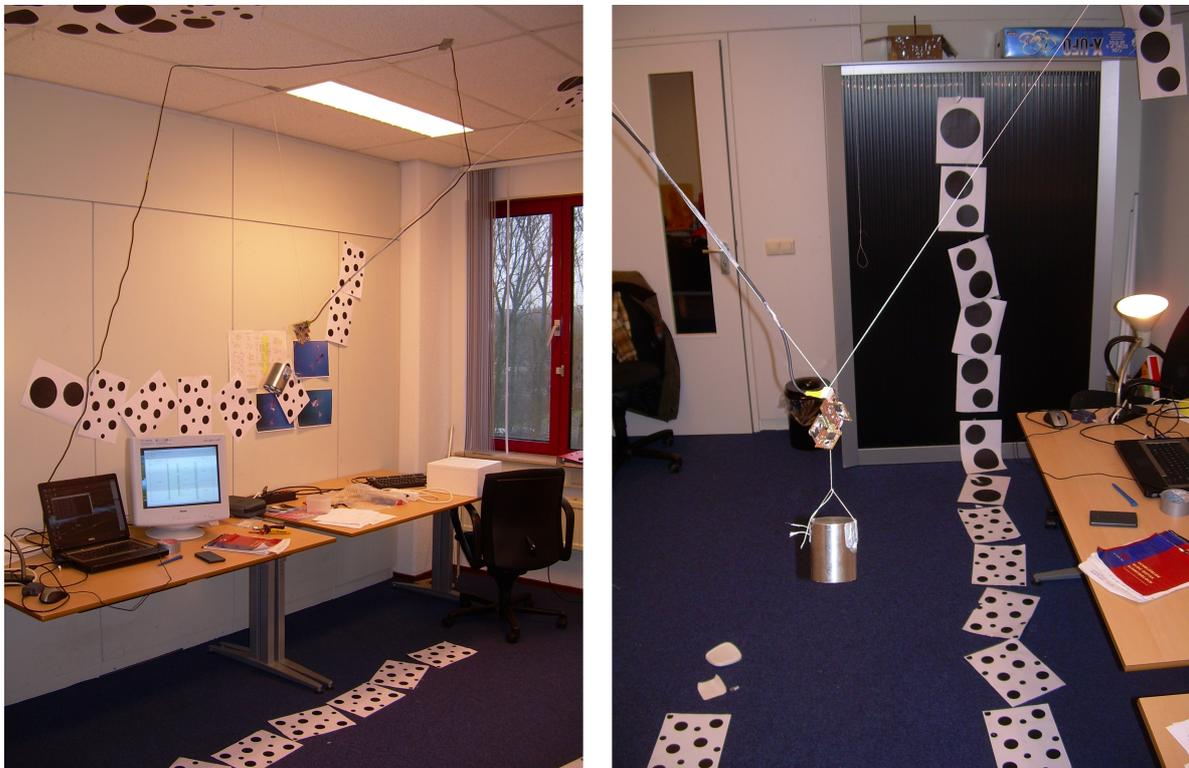
**Figure 9-1:** The office room at ASTI with the pendulum experiment setup. The dotted paper has been placed in the view of the sensors to enhance the texture and thereby tracking performance.
