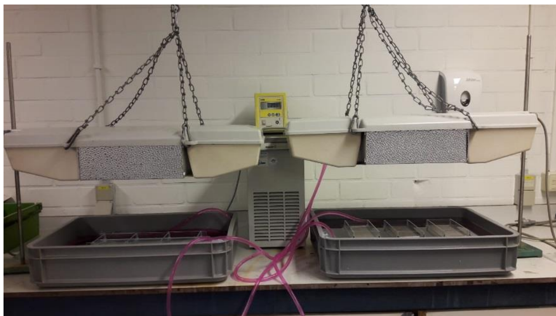
Figure 5.2. Experimental setup of the reactors used for the study of the inactivation of surrogate organisms under artificial light and dark conditions.
