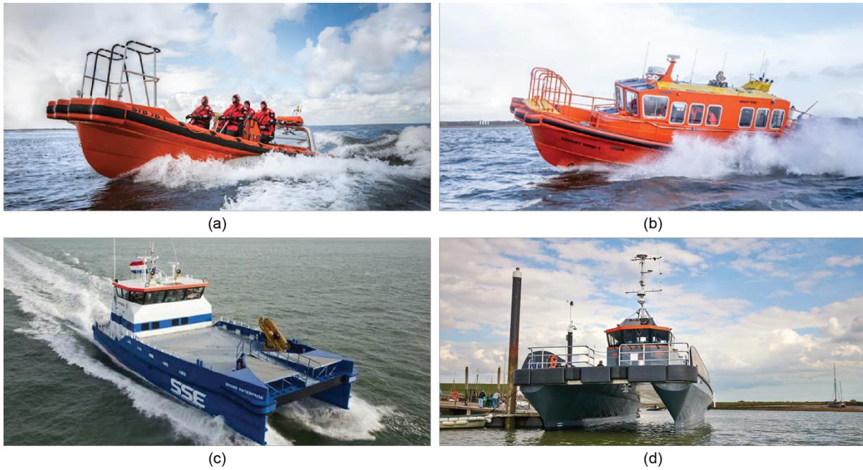
Figure 10: CTV configurations used on the offshore wind industry. (a) RIB, (b) monohull, (c) catamaran and (d) SWATH. Images adopted from ESVAGT (2017), Damen (2017) and CWind (2017).
