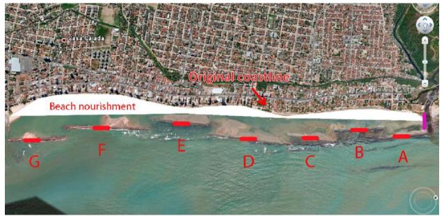
Figure 68: Sketch of alternative 1, breakwater lengths not on scale
