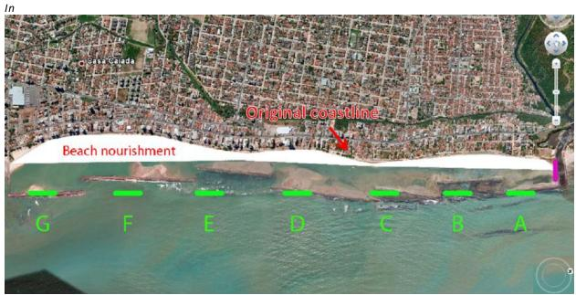
Figure 69 a sketch is made of the proposed changes for alternative 2. Note that the breakwaters in this figure are not to scale and the length are not representative, the image just shows the idea of alternative 2. The exact dimensions cannot be determined with the current information. Only an indication of the lengths will be given with the use of rules of thumb.
