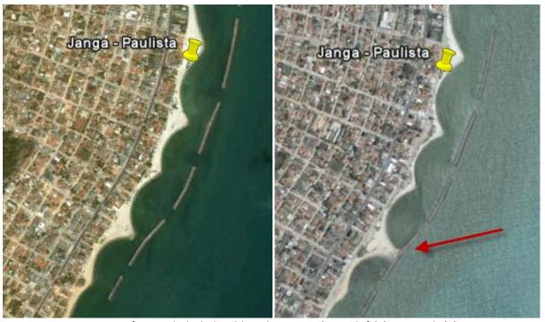
Figure 82: Formation of a Tombolo behind breakwater H (2003 left) (2007 right) (Image source: GeoEye, 2011)
