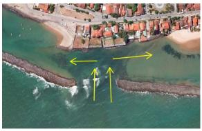
Figure 41: Indication of sedimentation and erosion in Fortim (Google Earth, 2009)
