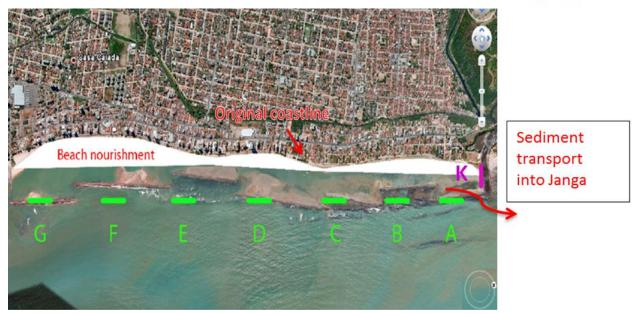
Figure 70: Sediment transport out of Casa Caiada
