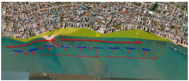
Figure 16: Expected main flow of the sediment with Alternative 2
