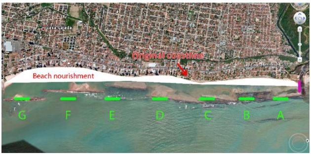
Figure 69: Sketch of alternative 2, breakwater lengths not on scale
