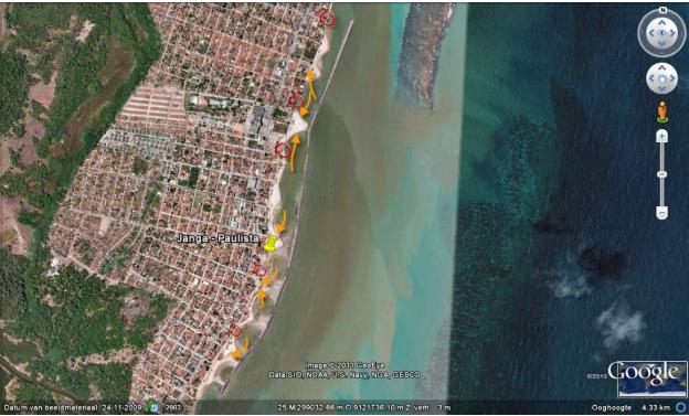
Figure 87: Reorganization of the shoreline due to breakwaters (Image Source: GeoEye, 2011) (The arrows indicate where sediment was moved from to form the tombolos) (The red dots indicate where revetments were built) (notice that the areas where sediment was taken from to form tombolos and where revetments have been built coincide? This is probably not coincidence)
