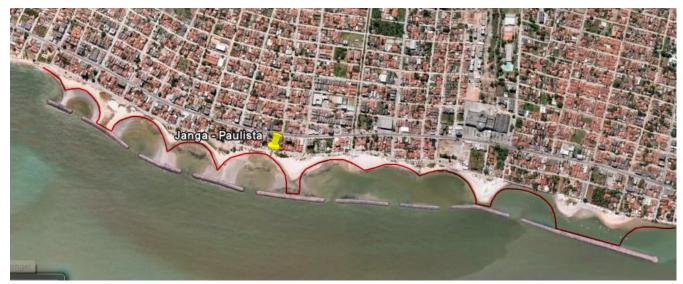
Figure 91: Prediction of what the shoreline should look like if there were no sediment deficit - The size of the Tombolo behind breakwater A is debatable but It will definitely be large (image: GeoEye, 2011)
