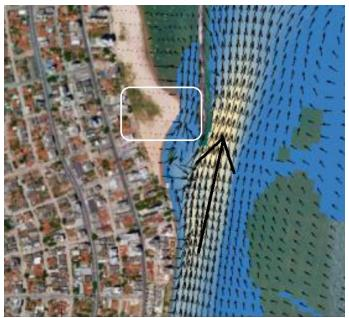
Figure 50: bypass phenomena of sediment transport in the Candeias area
