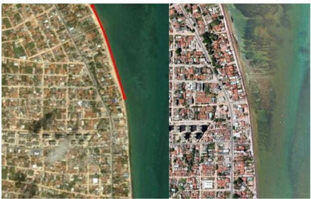
Figure 85: Revetments in the North (2003 left - small revetment) (2007 - Enormous revetment) (the extension of the revetment has been marked in red) (Image Source: GeoEye, 2011)
