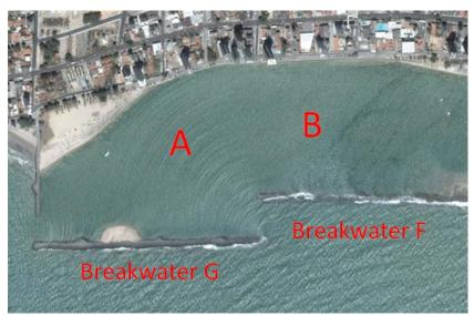
Figure 67 Diffraction patterns at breakwater F and G
