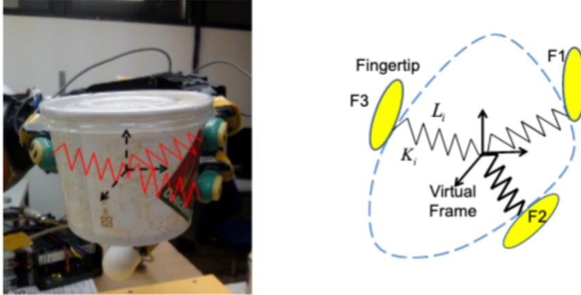
Figure 3.9: Left: The robot used by Li et al. [46] for their experiment with object-level impedance controllers. Right: A schematic showing the distribution of fingertips and the location of the defined *Virtual Frame*
