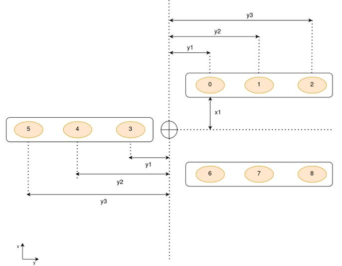
Fig. 5: The gripper configuration and the location of each sensor pad. The sensor mapping  $\mathcal{F}$  for each sensor pad  $i$ , ranging from 0 to 8, can be obtained by taking the distances of each pad from the center.
