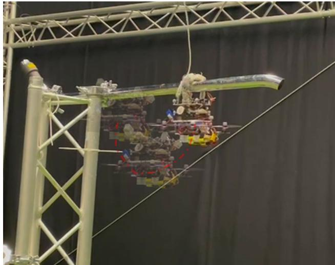
Fig. 1: The aerial manipulator using tactile-based navigation is depicted perching on an object.
