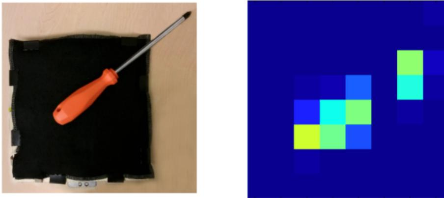
Figure 3.8: An example of how tactile feedback can be used to be able to perform tactile-based localization [15]. On the left, an image of a screwdriver on top of a tactile sensor pad is shown. While on the right the corresponding tactile image output is displayed.
