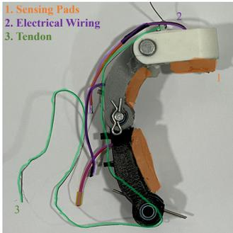
Fig. 3: The manufactured finger with sensing pads, electrical wiring and tendon.
