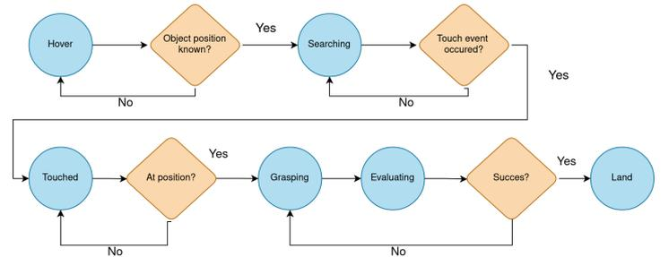
Fig. 6: Flowchart of the state machine
