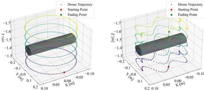
Fig. 7: Ellipse and zigzag search trajectories used in the searching state of the tactile state machine.
