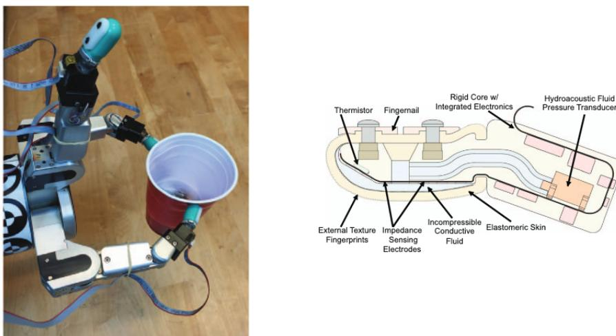
Figure 3.4: Left: A robotic hand with BioTac sensors attached to its fingertips [14]. Right: The internals of the BioTac sensor. [14]
