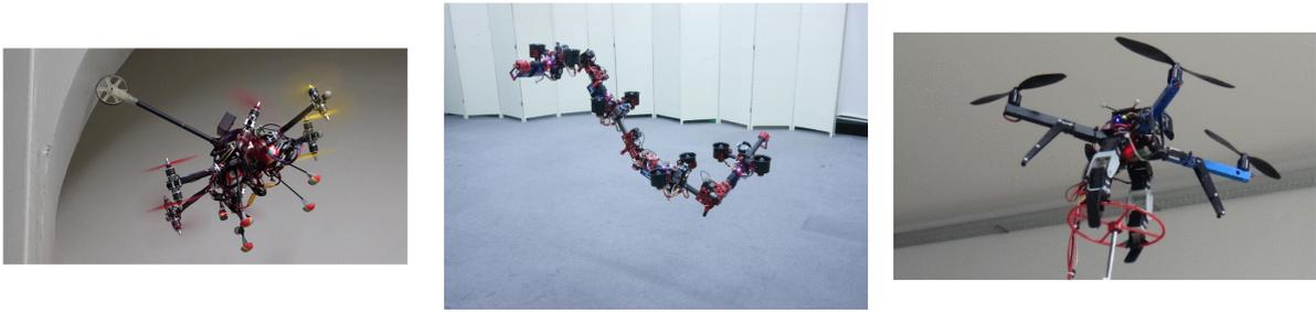
Figure 3.1: From left to right, An omnicopter developed by Bodie et al. [4] that is able to trace contours on a wall, a morphing drone developed by Zhao et al. which can be used for various applications [19] and a quadrotor manipulator developed by Korpela et al. that is opening a valve [10].
