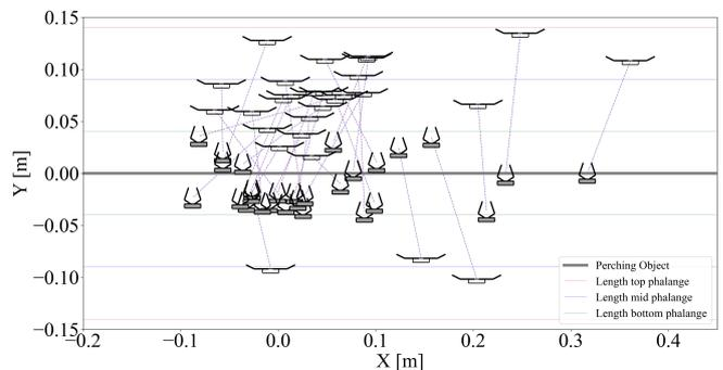
Fig. 12: The overall response pattern of the controller following a touch event is illustrated. The drone transitions to an “open” state upon detecting a touch event, and to a “closed” state when attempting a grasp. The depicted drone flight paths consistently converge toward the bar after a touch event. This data is derived from 28 individual trials involving varied offsets to the bar and searching trajectories.
