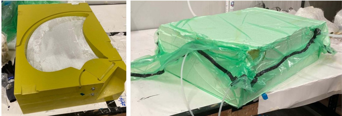
Figure 1. Production of a GFRP marine propeller. The left photograph shows the glass-fibre laminae inside the mould. The right photograph shows the mould under vacuum for the process of resin infusion. Photographs by W de Bles.
