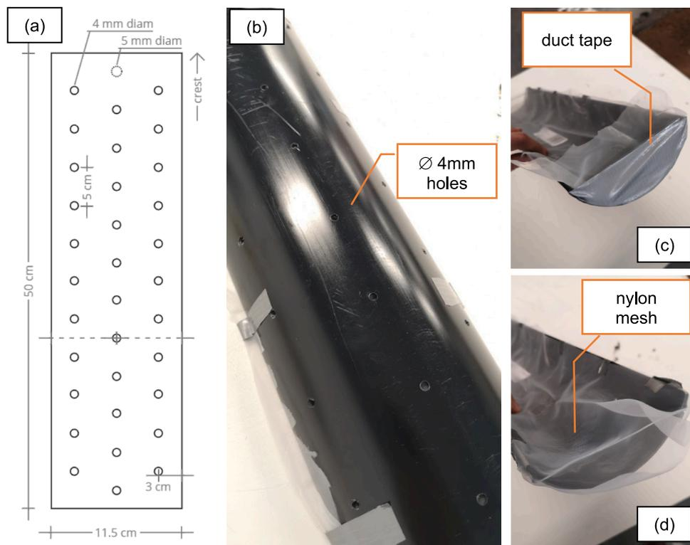
**Fig. 2.** Steps to build the columns (Part 1). (a) Sketch illustrating gutter dimensions and positioning of drilled holes allowing vertical percolation; (b) Perforated gutter; (c) Crest of column closed with duct tape avoiding soil loss; (d) Nylon mesh applied to avoid loss of soil fines and to allow data collection on subsurface flow.
