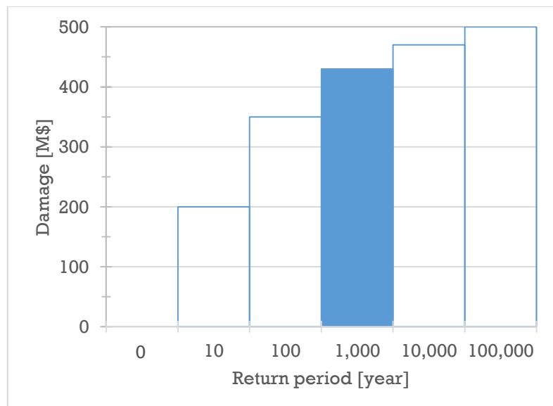
Figure 3-7: Storm asset damage illustration example
