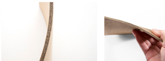
Image 17 Straw floor panels
