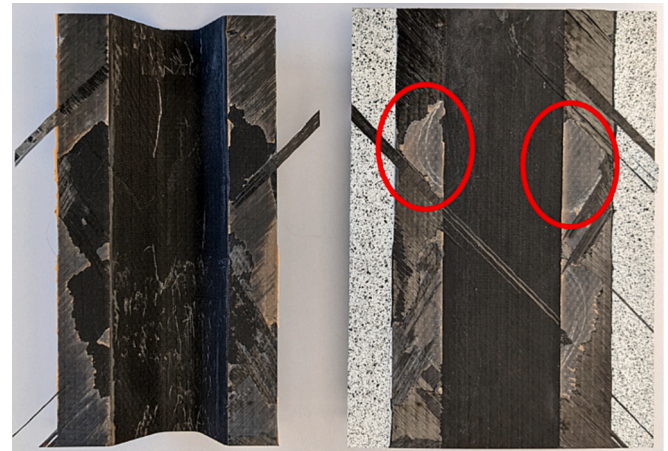
Fig. 13. Control1 Specimen Fracture Surface.
