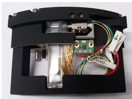
Figure 6.12: Sample Cell Unit Assembly with LL10.
