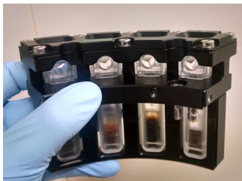
Figure 4.2: FOAM-C Sample Cell Unit Insert for the eBB.
