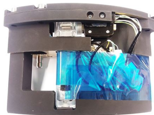
Figure 6.13: Sample Cell Unit Assembly with LL06.
