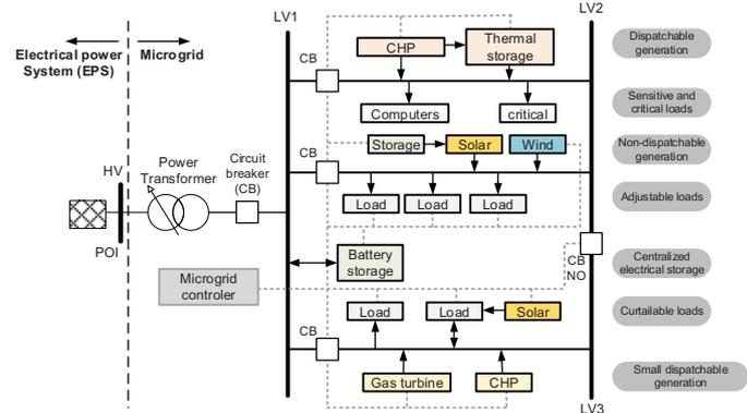
Figure 1. Diagram showing the structure of a  $\mu$ g and its components. Taken from [11] and the model has been modified for the very specific purpose of this paper.
