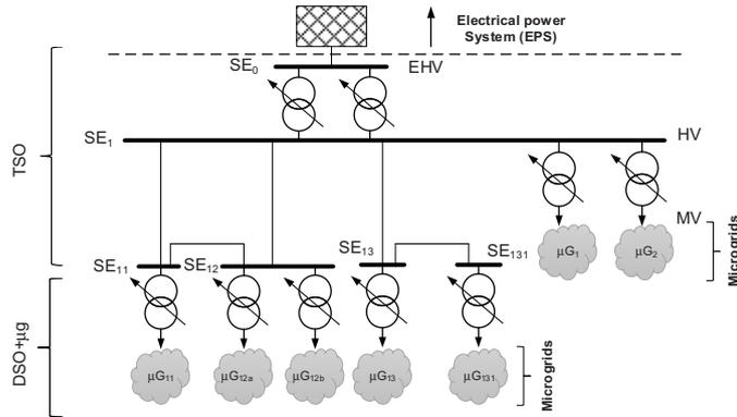
Figure 2. The general scheme of an EHV/HV/MV+μg system. TSO-DSO boundaries are shown.
