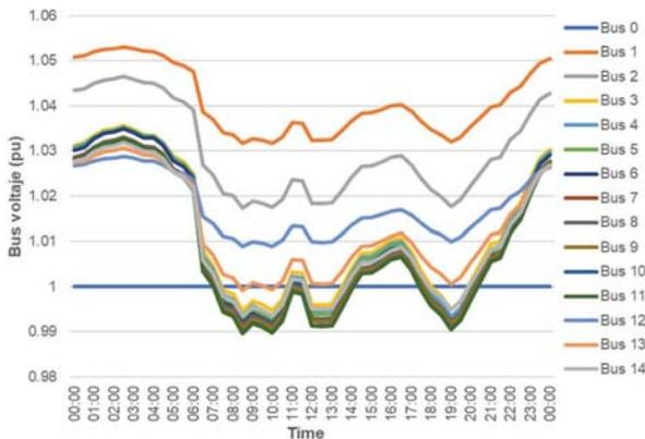
Figure 4. System voltages for the Base Case.
