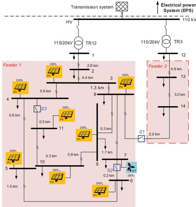
Figure 3. Test System: Single-line diagram depicting the European Distribution of the test system and the integration of DER.
