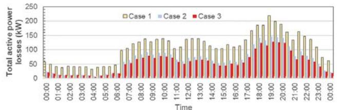
Figure 7. System losses comparison for Case 1, 2 and 3.
