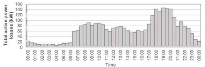
Figure 6. System losses for Case 2; Including of DER.
