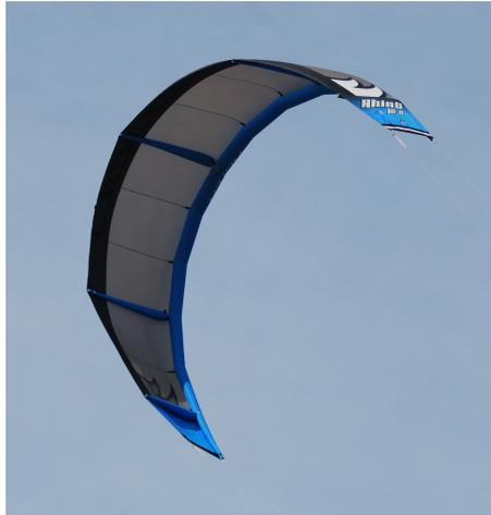
**Figure 9-1:** 'North Rhino' arc-shaped LEI Kite in flight
