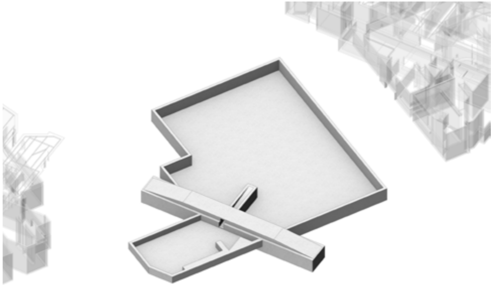
WATER TANK Reinforced concrete basement, 900mm
