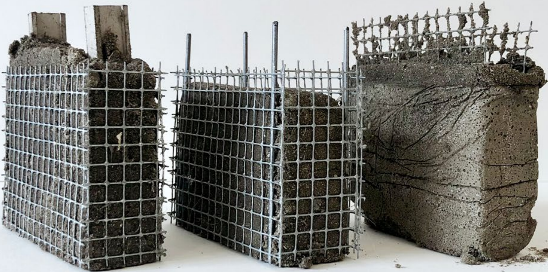
Wire mesh as the enclosed material Steel column as structure
