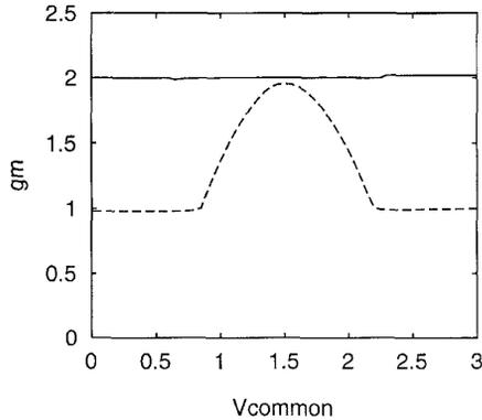
Fig. 2. Normalized  $g_m$  versus the common-mode input range for the rail-to-rail input stage with zener diode: - - - - rail-to-rail input stage without  $g_m$ -control, — rail-to-rail input stage with  $g_m$ -control.
