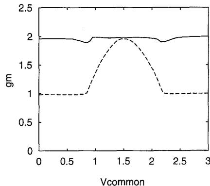
Fig. 6. Normalized  $g_m$  versus the common-mode input range for the rail-to-rail input stage with electronic zener diode: - - - - rail-to-rail input stage without  $g_m$ -control, —rail-to-rail input stage with  $g_m$ -control.
