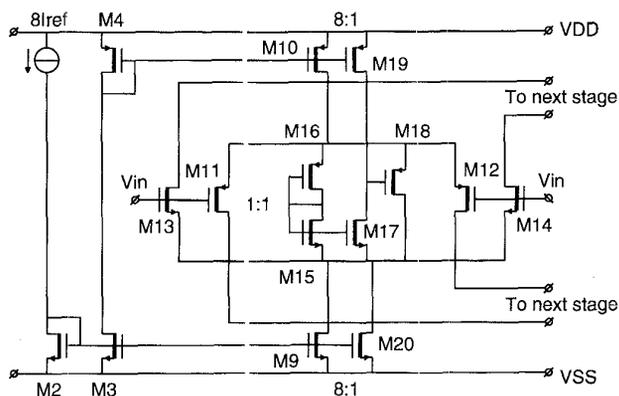
Fig. 5. Rail-to-rail input stage. The  $g_m$  is regulated by means of an electronic zener diode.
