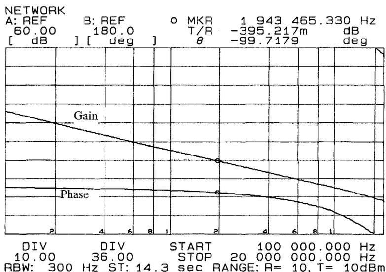
Fig. 9. Bodeplot of the compact operational amplifier. The  $g_m$ -control is implemented by means of an electronic zener diode.
