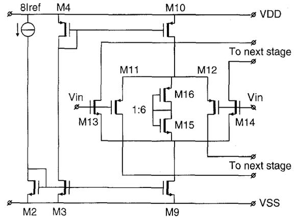
Fig. 3. Rail-to-rail input stage. The  $g_m$  is regulated by means of two complementary diodes.
