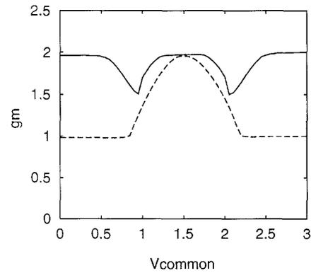
Fig. 4. Normalized  $g_m$  versus the common-mode input range for the rail-to-rail input stage with two complementary diodes: - - - - rail-to-rail input stage without  $g_m$ -control, — rail-to-rail input stage with  $g_m$ -control.
