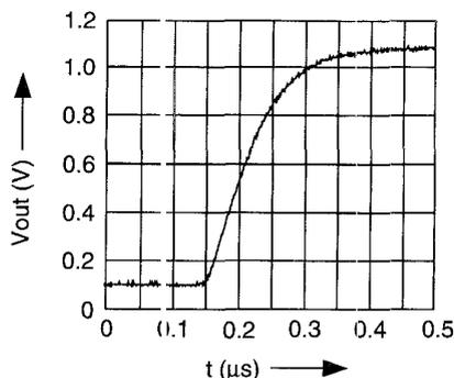
Fig. 10. Step response of the compact operational amplifier ( $V_{step} = 1$  V). The  $g_m$ -control is implemented by means of an electronic zener diode.
