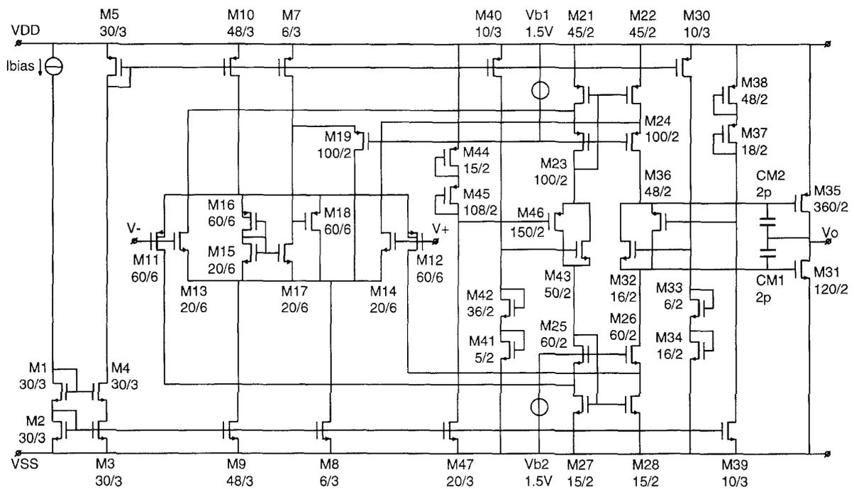
Fig. 7. Realization of the compact operational amplifier. The  $g_m$ -control is implemented by means of an electronic zener diode.
