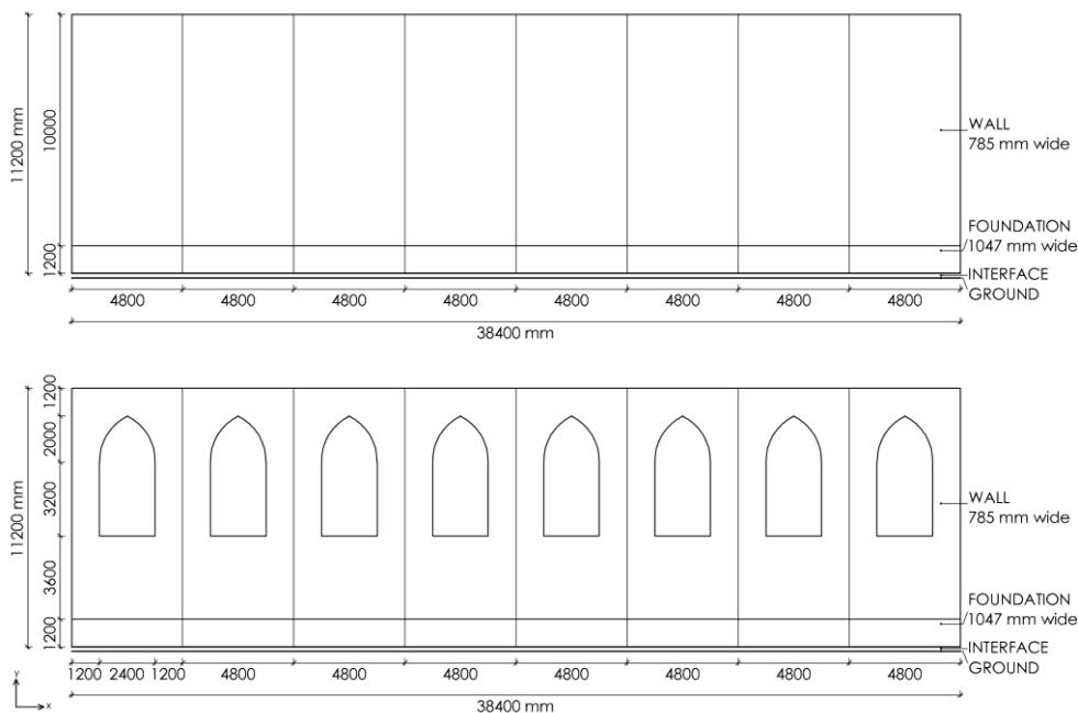
Figure 7.1: Geometries of the blind wall (top) and the wall with openings (bottom), with reference to dimensions.
