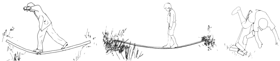
Figure 2.1: Lack of strength, lack of stiffness and lack of stability. Illustrations taken from Beranek [1997].
