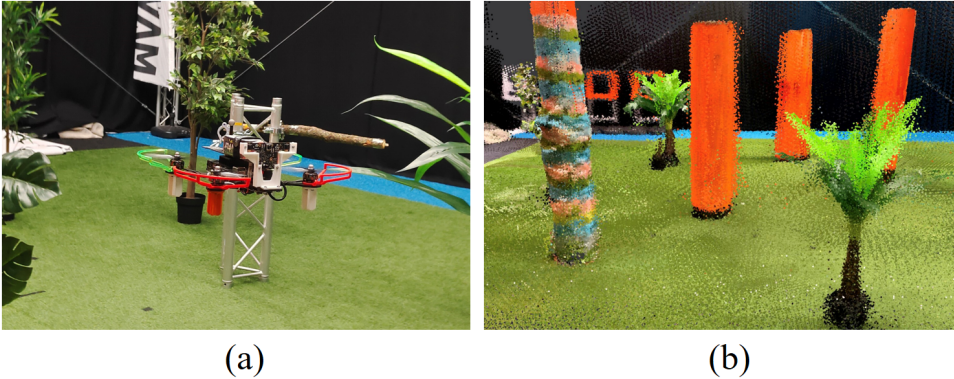
Figure 2.7: (a): Experiment platform for real world tests. (b): High-precision point cloud map built by a lidar sensor.
