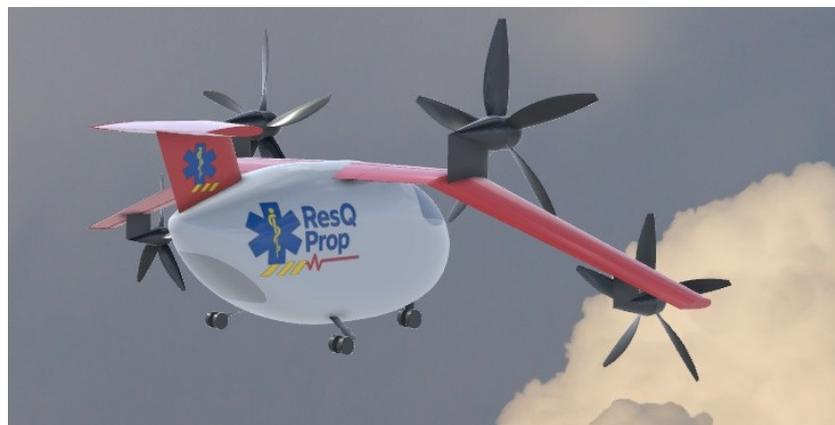
**Figure 17.1:** *ResQProp in cruise configuration*
