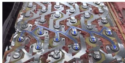
Figure 8.10: Tesla Busbar[41]
