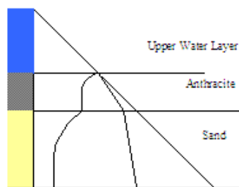
Figure 2-16 – Pressure curves in a filter bed (Miska-Markus, 2009)
