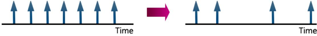
**Figure 2-15:** Periodic (left) and aperiodic (right) sampling [22].
