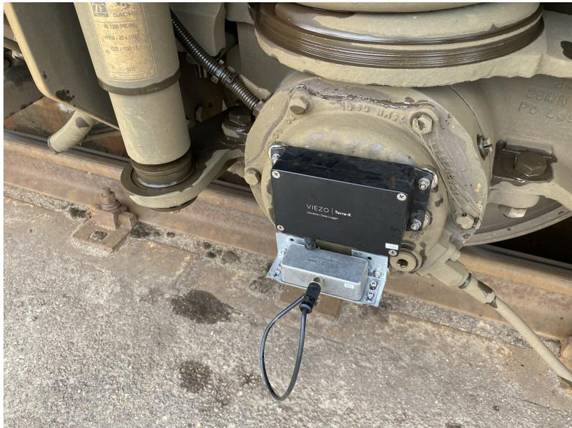
Figure 1-2: Railway energy-harvesting device made by Viezo [17].
