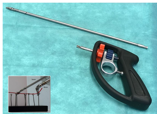
Fig. 8 SATA grasper handle detached from shaft assembly. Window image: 5 mm and 8 mm SATA instruments in action during a wire chasing training task
