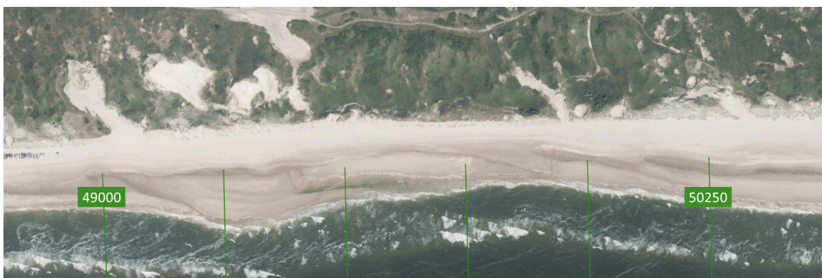
Figure 4.18: Aerial picture of the dunes of cluster 2. Transects directly crossing a blow-out are highlighted and the number shows the alongshore RSP coordinate in metres. Picture obtained from Coastviewer (Deltares, 2018).
