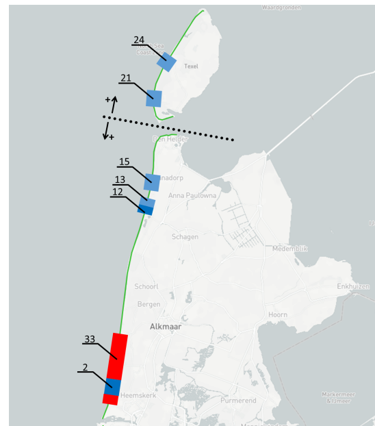
Figure 4.7: Map of the research area that shows the locations of the selected clusters. The RSP line is shown in green and the arrows indicate the positive direction of the RSP coordinates.
