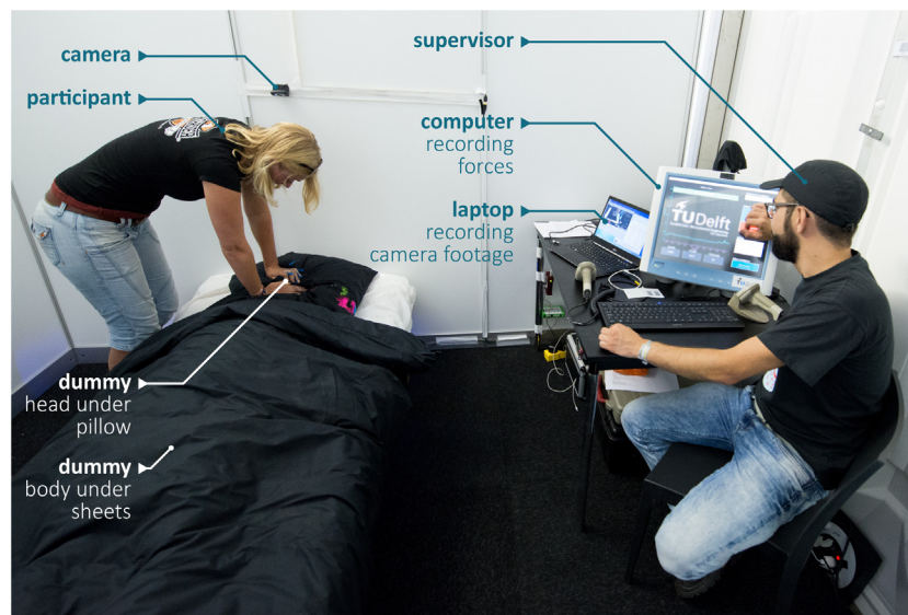
Fig. 1. Overview of the setup used for the smothering experiment. The wooden dummy head rested on a force measuring unit, which is described in Fig. 2.
