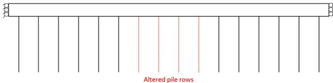
Figure 5.2: Non-uniform pile degradation will be simulated by altering pile row properties in the finite element model.
