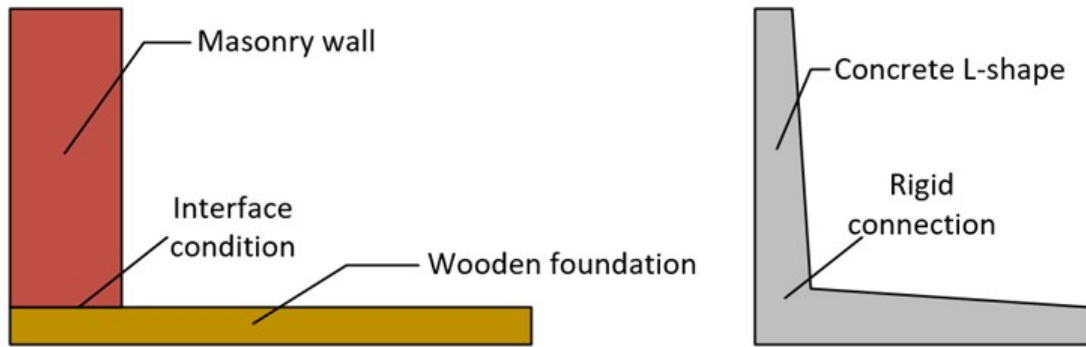
Figure 3.19: Notice the L-shape in the historical quay wall and a modern concrete cantilever wall (representation).
