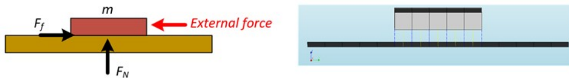
Figure 4.19: Example case to verify the Coulomb Friction Model and its representation in DIANA FEA.
