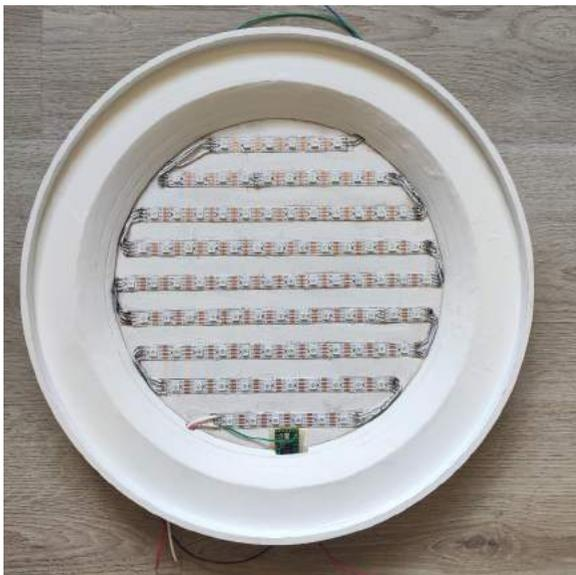
Figure 63 - Final model with LED matrix
