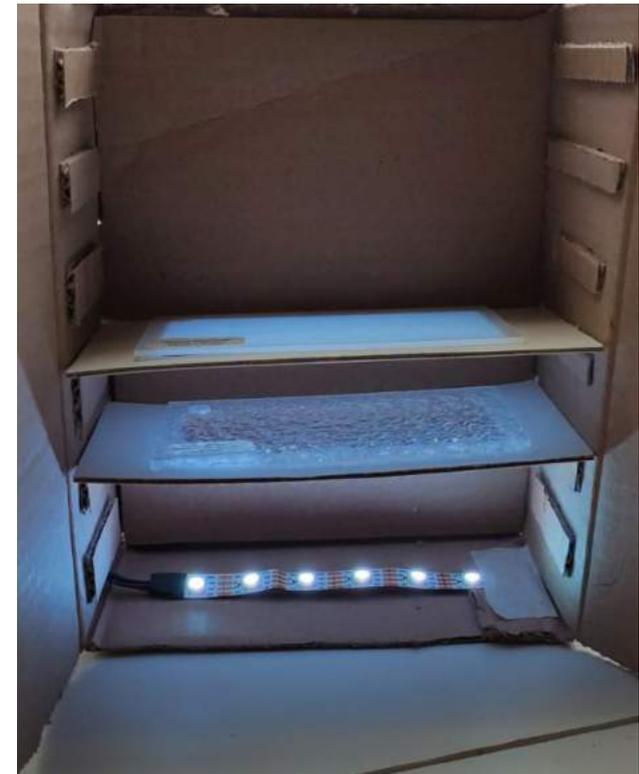
Figure 52 - Test setup for light diffusers
