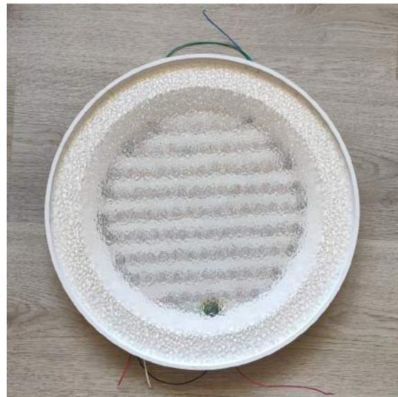
Figure 64 - Final model structure diffuser
