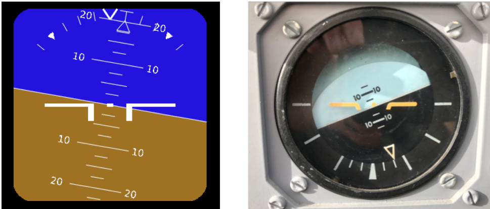
Figure 4.1: Left is the moving horizon type AI used in the simulator experiment, showing a left turn. The AI is a simplified version of the AI used in large jet airliners. Right is the AI used in the in-flight experiment, showing a right turn.
