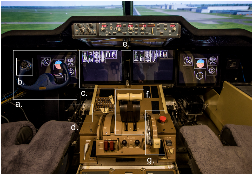
Figure 6.1: The flight deck as used in the experiment. Visible are: a. control column and primary flight display; b. pitch trim controls; c. engine display; d. rudder pedals; e. gear lever; f. throttle lever; g. flap lever.
