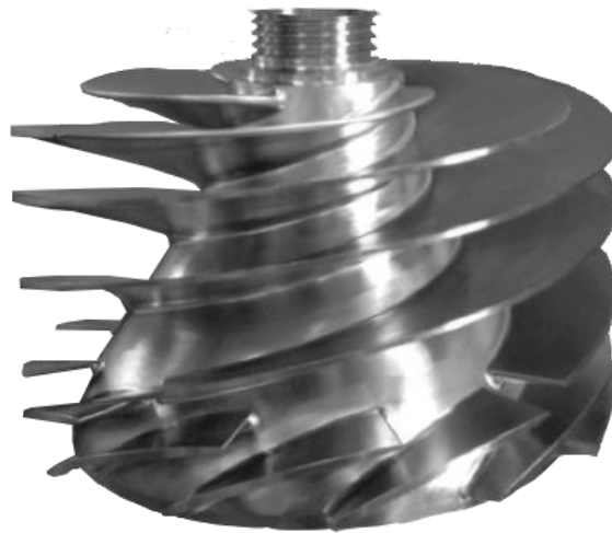
Figure 3 – Geometry of the 4-bladed MIT test inducer is based on the SSME LPOP inducer [34]
