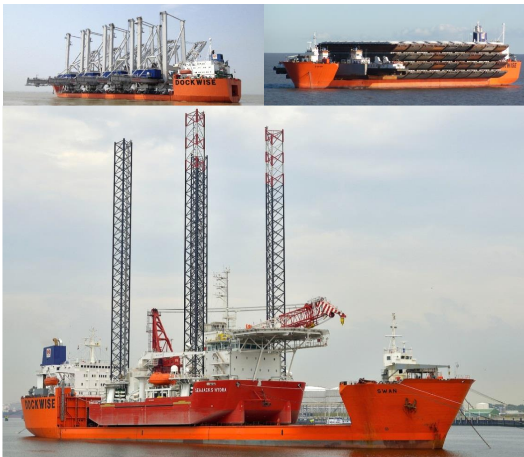
Figure 2-3: S-class loaded with CCR (top left) Liftboat (centre) and Barges (top right)
