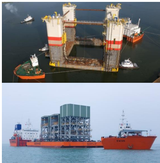
Figure 2-2: The S-class loaded with a TLP-hull ((top)), and modules on an FSP ((bottom))
