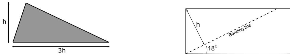
Figure 6. Schematic layout of VG model used (left) and fabrication method from a rectangular metal sheet (right).
