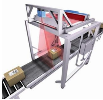
FIGURE 27 AUTOMATED (VOLUME)SCANNING AND WEIGHING OF ITEMS
