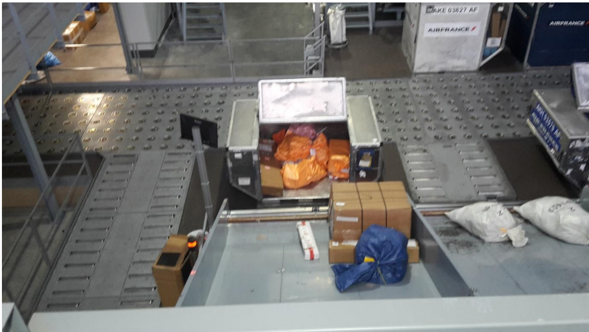
FIGURE 3 DESTINATION CHUTE ULD BUILD UP WITH CARGO AT SODEXI HUB, PARIS
