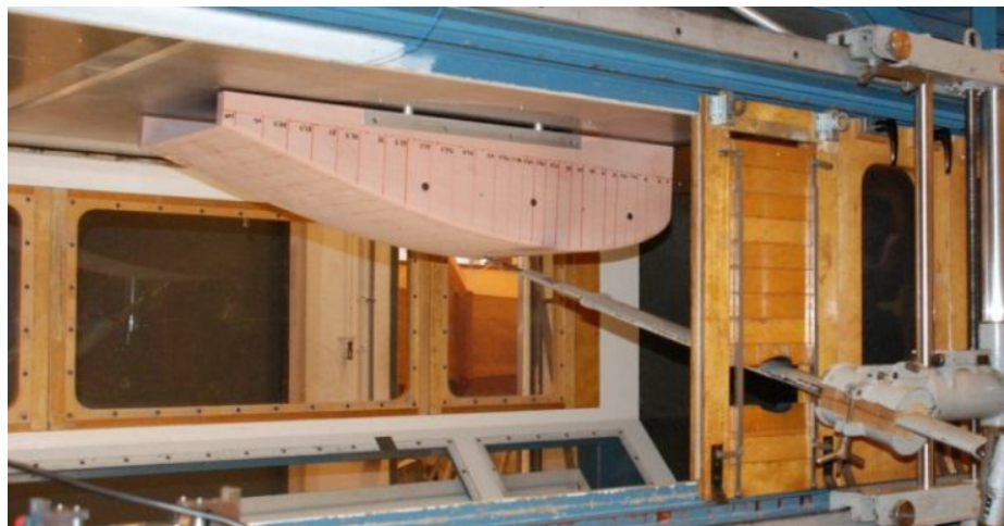
Figure 3. The AeroCity wind tunnel model suspended upside down in the test section of the Low-Turbulence Tunnel (LTT).
