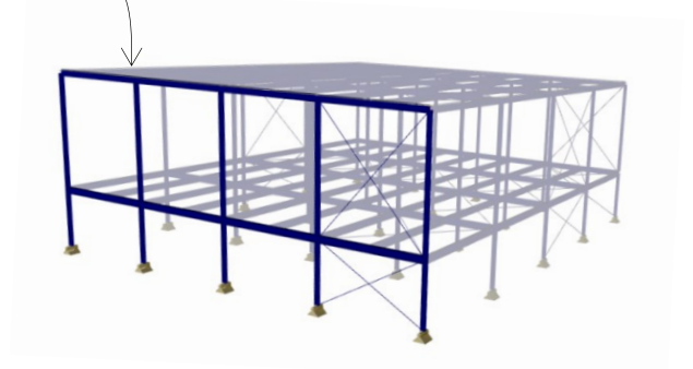
Figure 47: Demountable Scalable design conceptual structural overview: Side views, floor plan, and stability system.
