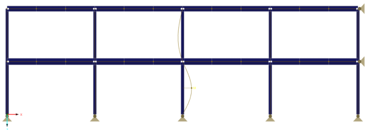
Figure B- 8: Eigen value analysis' first buckling mode shape and the associated critical load factor of DA01.
